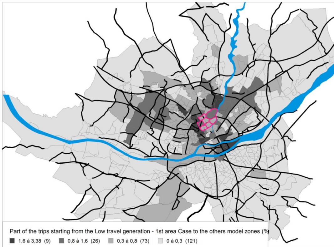
Figure 52 Spatial distribution of the destination zones for the modified trips - Case 2 – Sub-Case 1 – Low travel generation – 1st area (Stimulus 1)
