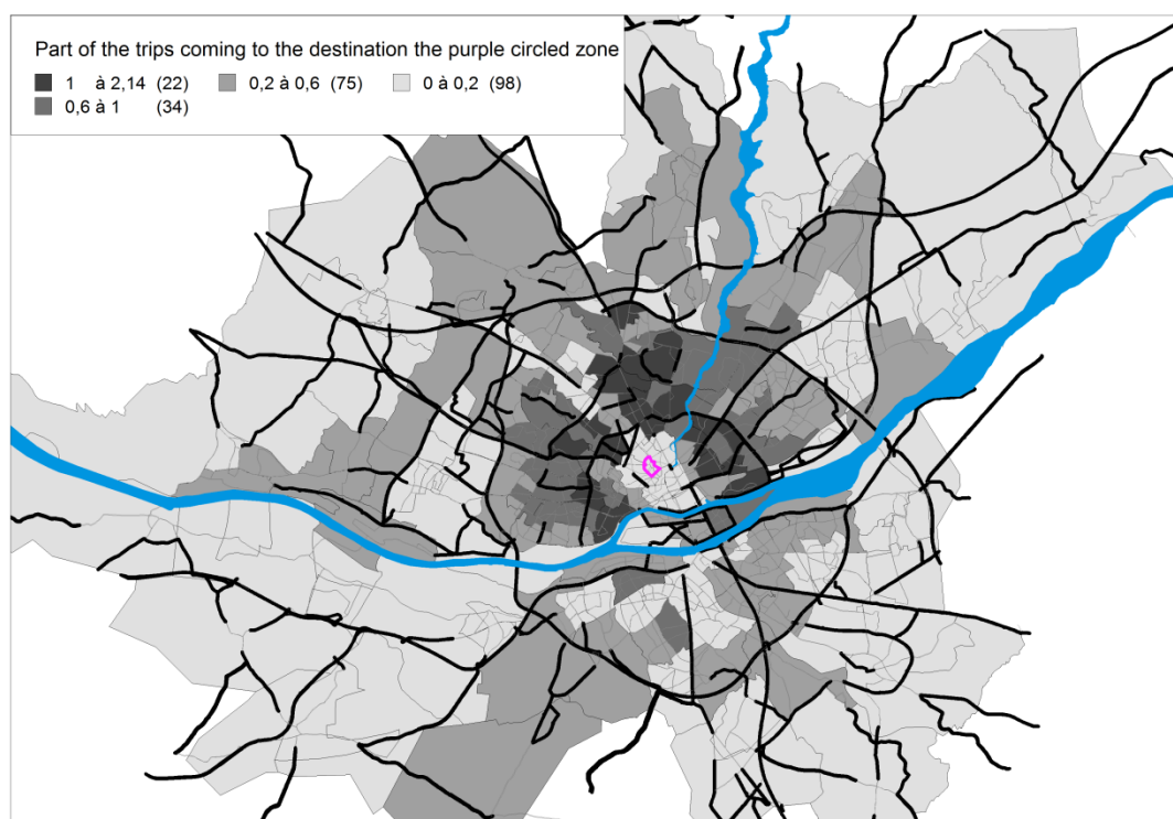
Figure 64 Spatial distribution of the origin zones for the modified trips – Case 3 – Sub-Case City Center (Stimulus 1)
