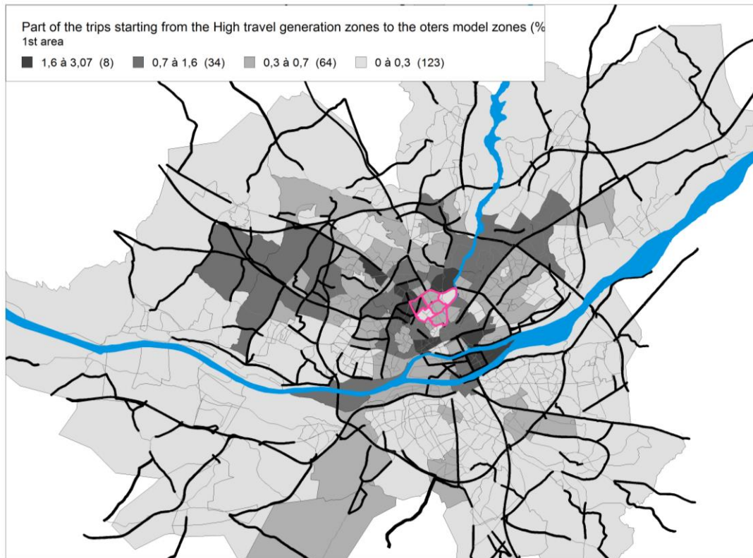
Figure 56 Spatial distribution of the destination zones for the modified trips - Case 2 – Sub-Case 2 – High travel generation – 1st area (Stimulus 1)
