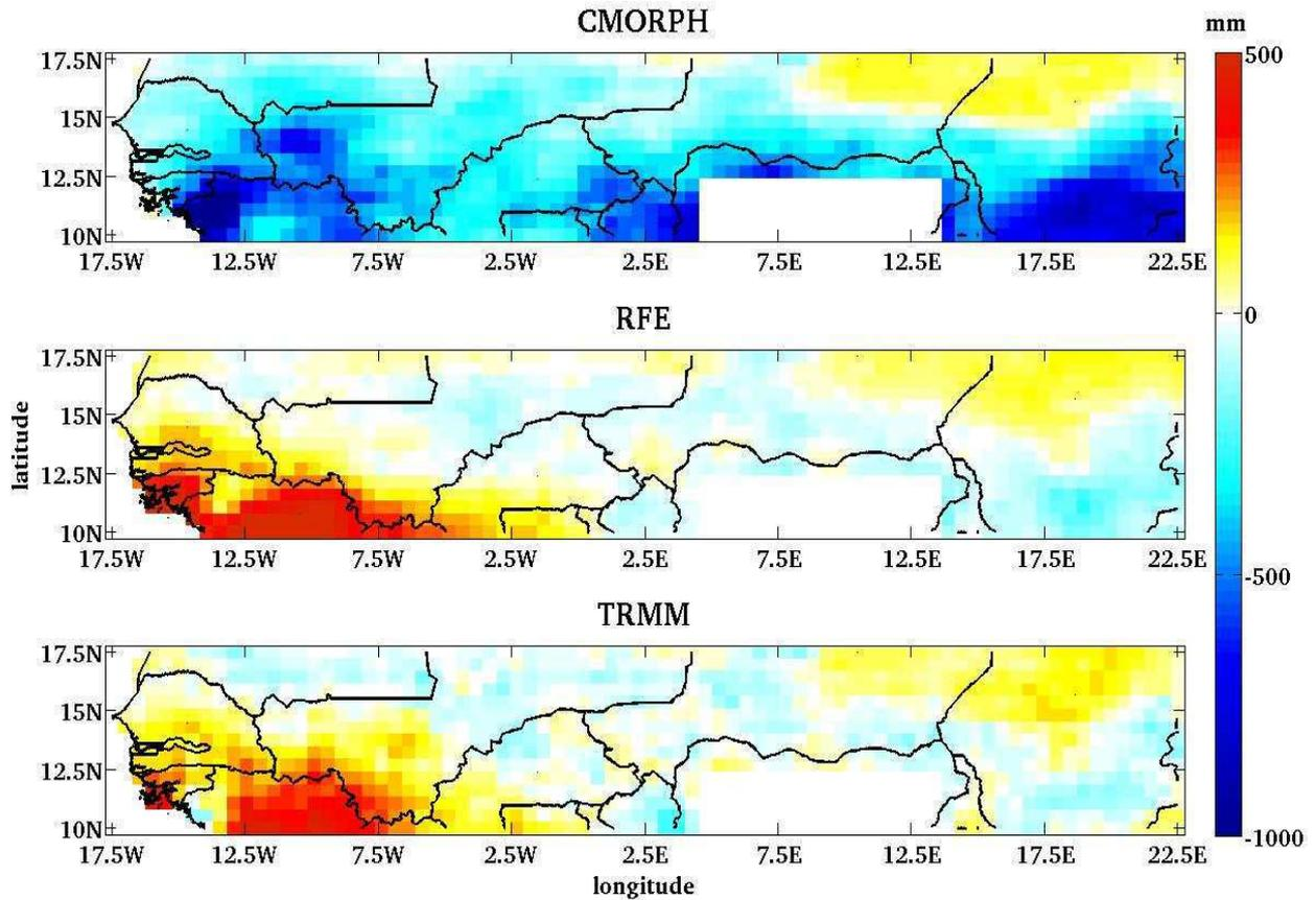
*Figure 2-20 : Mean annual differences in precipitation amount over the rainy season (May to October) averaged over the 2004-2007 period between the 3 satellite derived precipitation products and the kriged rain gauge data.*
