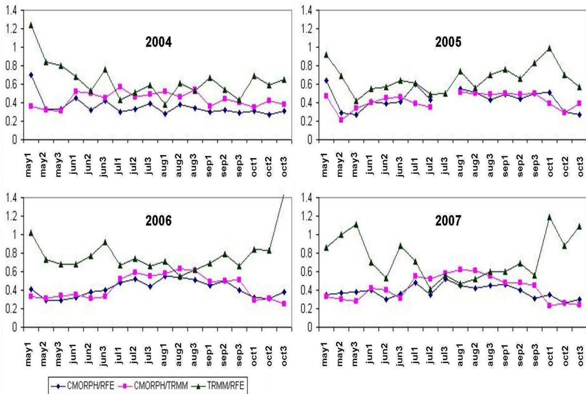
**Figure 2-18** : Slopes of the linear regression of the rainfall amount for couples of satellite derived precipitation products during the rainy season for the period 2004 to 2007 and for the area 10°N to 20°N; 20°W to 35°E. Missing values (e.g. end of July 2005) correspond to missing satellite data.
