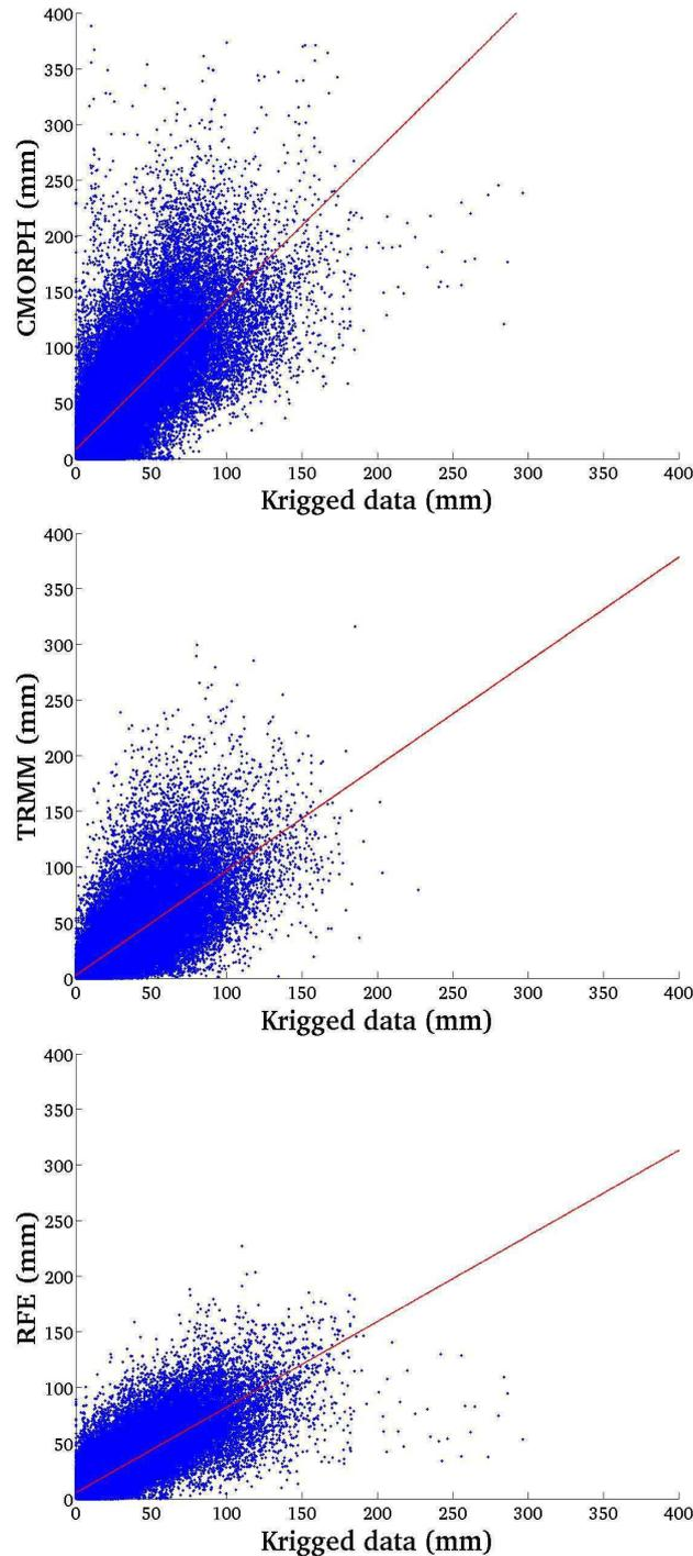
**Figure 2-19 :** 10-days rainfall estimates (mm) of CMORPH (top), TRMM3B42 (middle) and RFE2.0 (bottom) versus kriged rain gauge data for the rainy seasons (May to October) 2004 to 2007 and for the area  $10^{\circ}\text{N}$  to  $17.5^{\circ}\text{N}$ ;  $17.5^{\circ}\text{W}$  to  $22.5^{\circ}\text{E}$ .
