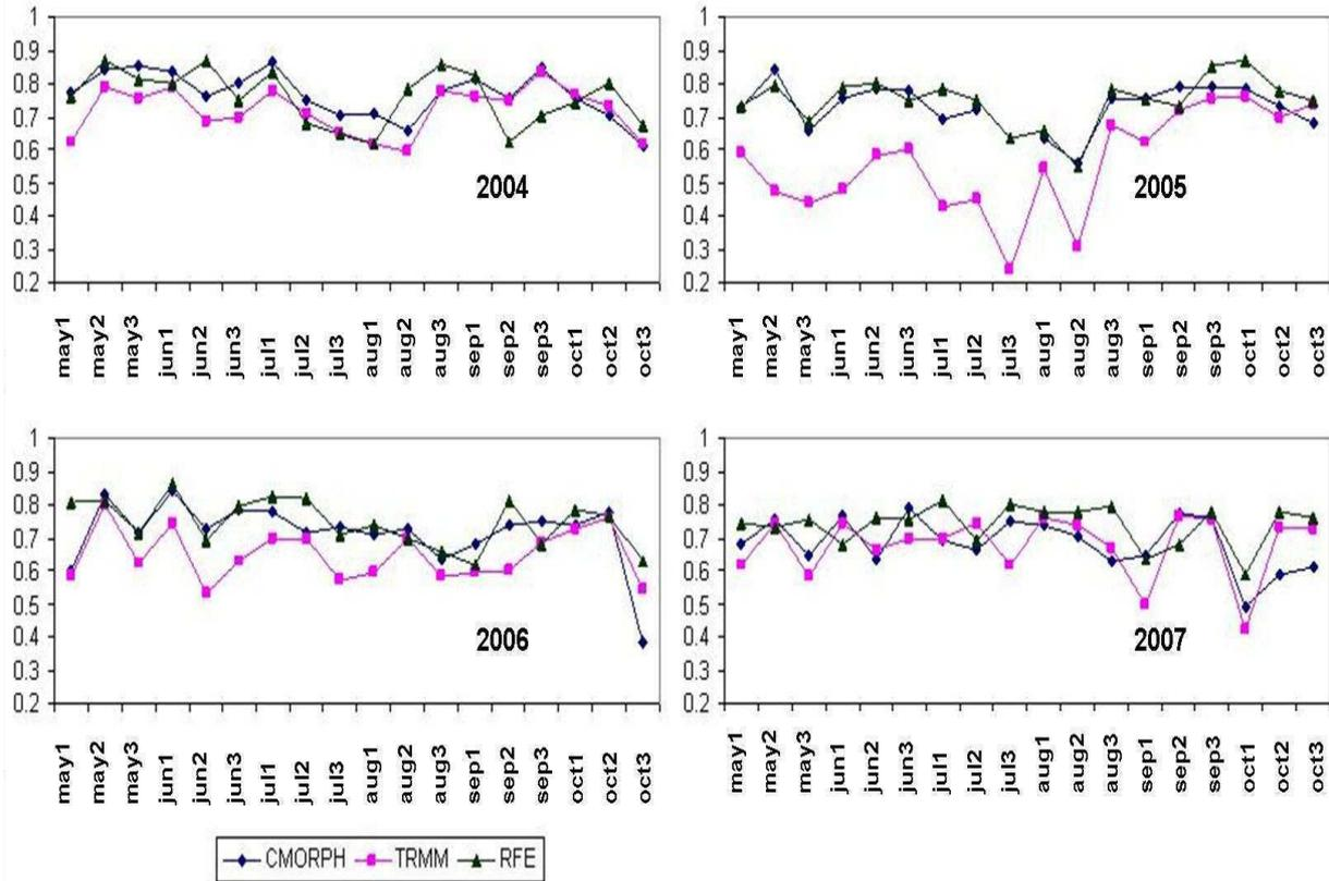
**Figure 2-11** : Correlation coefficients during the rainy season (May to October) of 2004 to 2007, between the three satellite derived precipitation products and spatially interpolated gauges-measurements. Correlation coefficients are computed by decade over the area  $10^{\circ}\text{N}$  to  $17.5^{\circ}\text{N}$ ;  $17.5^{\circ}\text{W}$  to  $22.5^{\circ}\text{E}$ .
