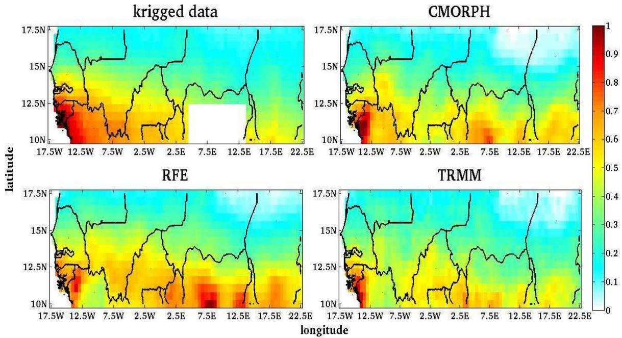
**Figure 2-10 :** Normalized cumulated rainfall during the rainy season (May to October) 2004 to 2007, for the kriged gauges measurements and for the three studied satellite-based products. Interpolation not taken into account over Nigeria (white box: no gauges measurements available).
