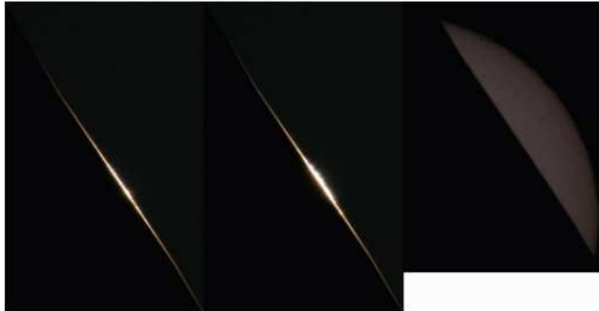
Fig. 4. Fringes with the occulted rising Sun while focusing on the wall at 150 m and a 0.25 ms exposure at 200 iso without ND; the solar disk at the same scale with a ND 3.8 and 5 ms exposure.
