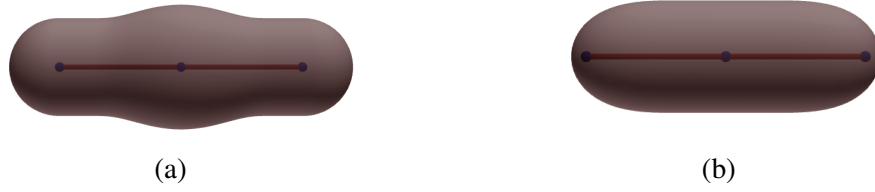
FIGURE 1.5 – Blending by summation of two primitives : distance primitives (a) create a bulge while convolution surfaces (b) seamlessly blend.
