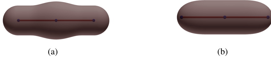
FIGURE 1.5 – Blending by summation of two primitives : distance primitives (a) create a bulge while convolution surfaces (b) seamlessly blend.
