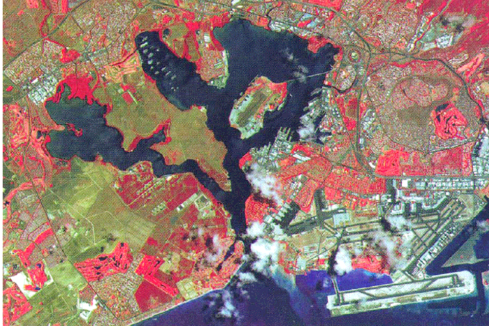
Picture 1.3: An image remotely sensed in two visible and one NIR band displayed and printed in one RGB colour space
