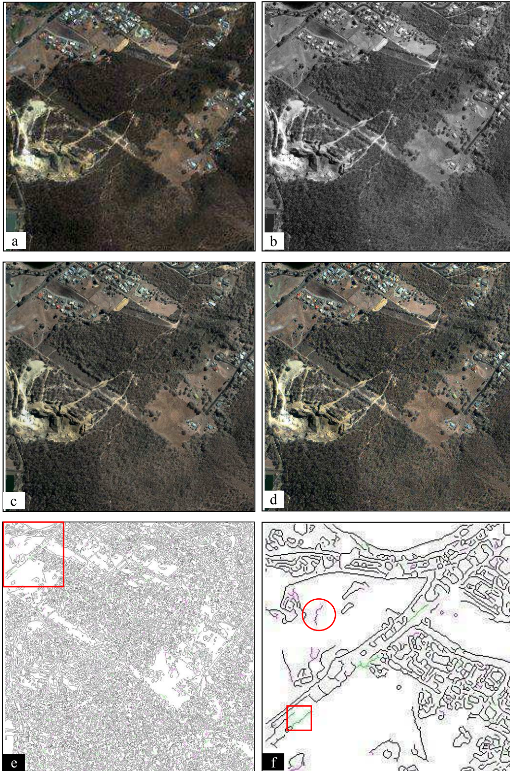
Figure A.2 Set 2, (a) low-resolution RGB image. (b) Corresponding Pan image. (c) Fused result using Bicubic interpolation. (d) Fused result using ICBI interpolation. (e) Edge information visualized as RGB image, where channels R, G and B correspond to edges extracted from images shown in (b), (c) and (d) respectively. (f) An area of (e).
