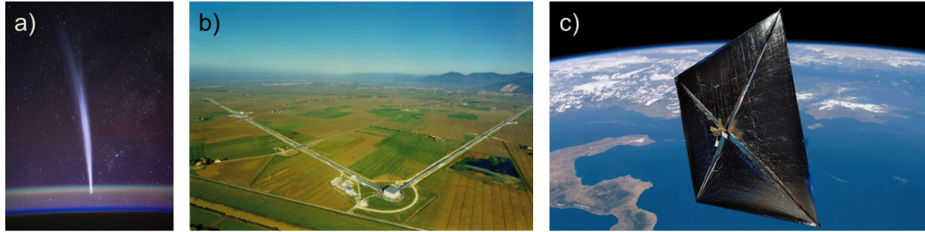
Figure 1: Three large scale systems sensitive to radiation pressure. (a) Comet's tail bending away from the sun. (b) VIRGO, a kilometer-sized Michelson interferometer located in Italy [2]. (c) NASA's NanoSail-D spacecraft (artist rendering) makes use of radiation pressure, in this case for space travel. Even though the acceleration provided by the solar radiation is feeble, it accrues over long periods of time, potentially allowing for fast and fuel-free space travel [3].
