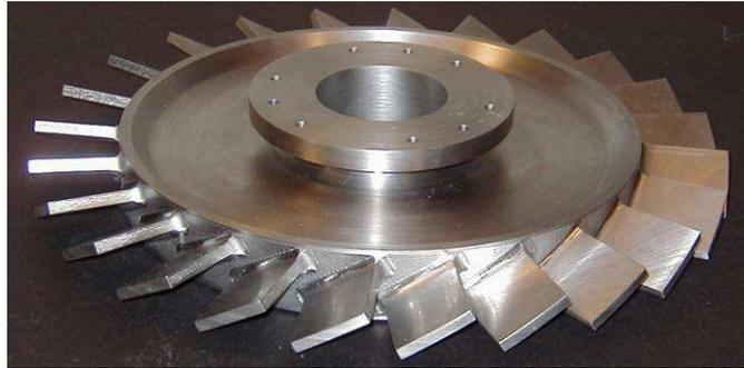
Figure 2.4: Picture of 24 blade validation rotor.
