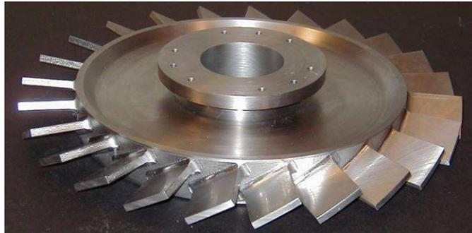
Figure 4.19: Actual 24-blade validation blisk used in the experiment.
