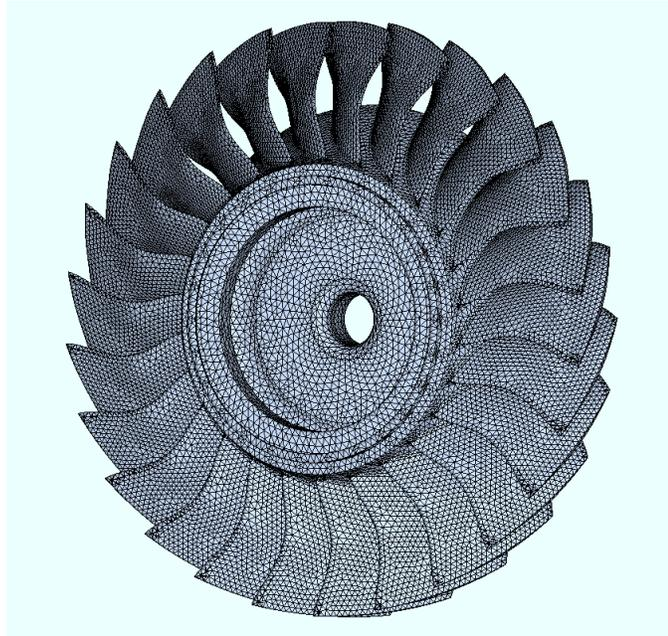
Figure 2.21: Finite element model of the NASA bladed disk.
