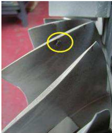
Figure 2.29: The mass (lead) added to tip of a blade of the NASA bladed disk.
