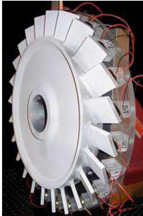
Figure 3.2: Actual bladed disk used in the experiment, shown with the acoustic excitation system.
