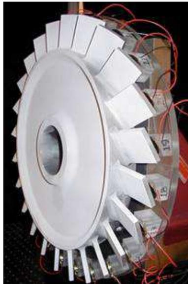
Figure 2.3: Bladed disk set up with blisk system installed.
