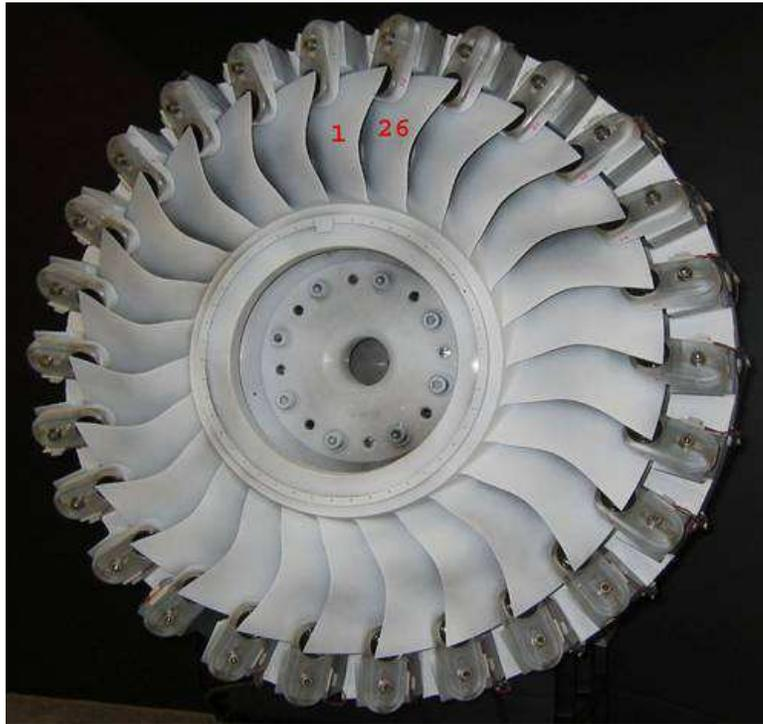
Figure 2.20: The NASA bladed disk mounted with speakers.
