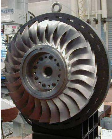
(a) Attach NASA bladed disk to fixture flange in the workshop
