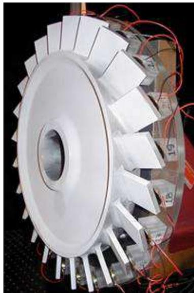
Figure 4.20: Validation blisk shown with the acoustic excitation system.
