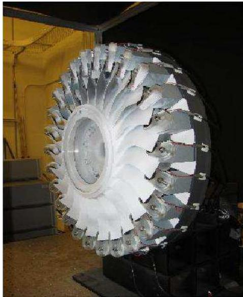
(c) Mount speaker behind each blade on the anti-vibration table, connected to signal generator
