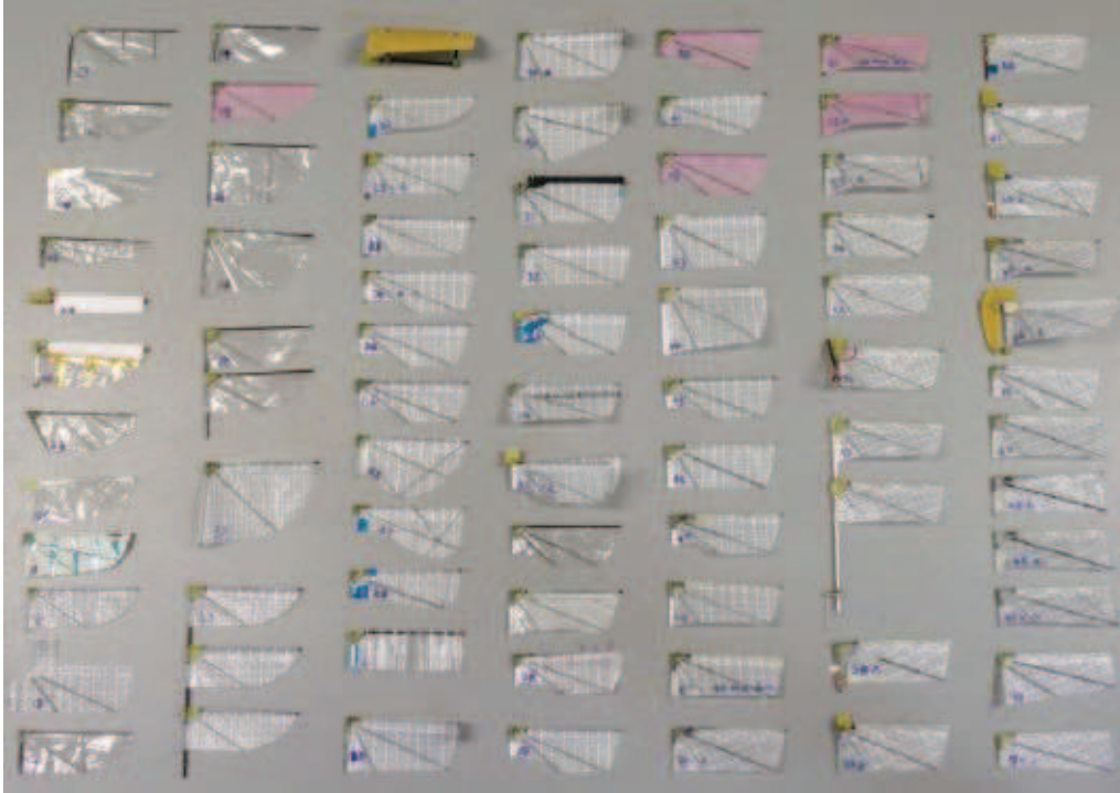
Figure 6.6: Set of wings used by Aerovironment to design successfully their NAV (Source: Keennon [2012]).
