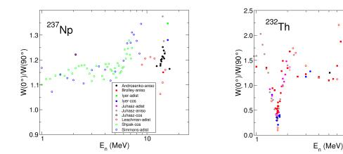
Figure 1.1: Existing measurements of the anisotropy of fission fragments for <sup>237</sup>Np (left) and <sup>232</sup>Th (right). For sake of clarity the uncertainty is not reported, the dispersion of the points is an indication of the actual uncertainty.
