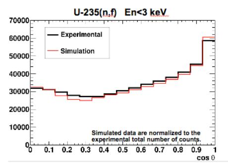
FIGURE 5.5: Detection efficiency for  $^{235}$ U and  $E_n < 3$  keV (isotropic) versus angle between fission fragment and the beam direction. Comparison between experiment and simulation [4].
