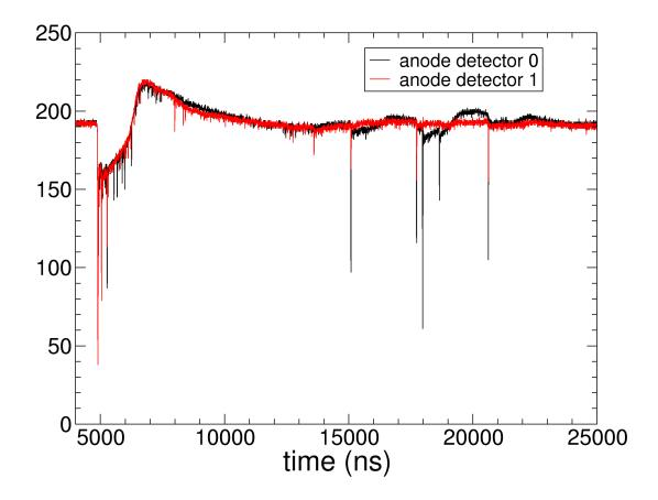
FIGURE 4.1: Expanded view of the beginning of a frame recorded on anodes 0 and 1 surrounding the  $^{235}\mathrm{U}$  target. Each frame is a series of amplitude measurements every 2 ns
