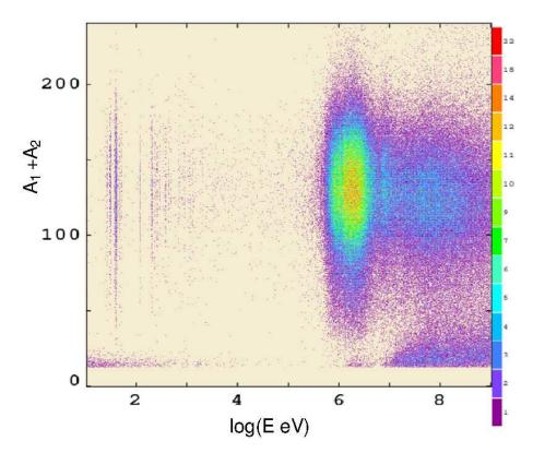
Figure 4.13: Distribution of the sum of anode amplitudes in detectors around the  $^{237}$ Np target, as a function of the neutron energy.
