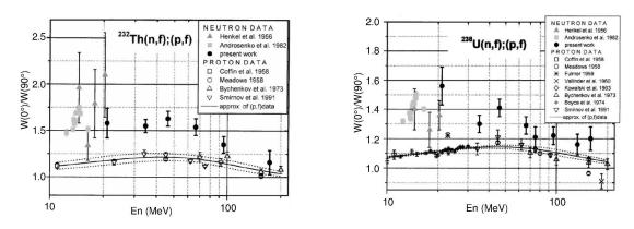
Figure 1.2: Comparison of anisotropy for neutron- and proton-induced fission for  $^{232}$ Th (left) and  $^{238}$ U (right) [1].
