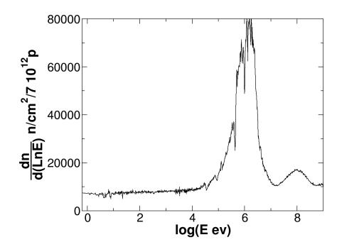
FIGURE 3.4: Phase I n\_TOF neutron fluence measured with  $^{235}\mathrm{U}$  and PPACs . The last collimator was 8 cm in diameter.
