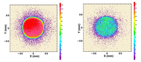
FIGURE 4.26: Distribution of emitting points on the <sup>235</sup>U target (left) and one of the <sup>232</sup>Th targets (right).
