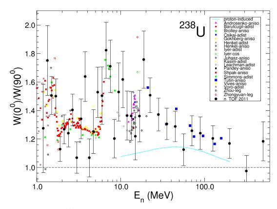
FIGURE 6.8: <sup>238</sup>U anisotropy with the old measurements, n\_TOF data and proton induced data
