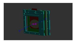
FIGURE 3.10: View of a 2 PPAC+target ensemble tilted by 45° against the neutron beam direction.
