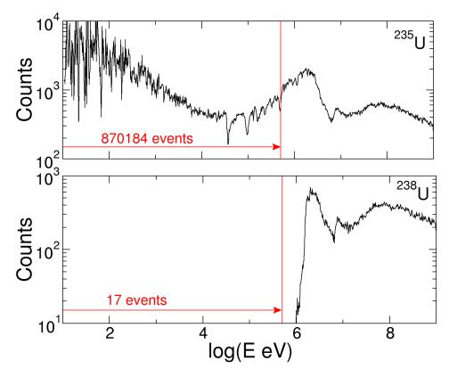
FIGURE 4.14: Energy spectrum of counts for the <sup>235</sup>U target and its <sup>238</sup>U neighbor. The red vertical lines are located at 0.5 MeV and indicate the limit of integration of counts indicated in red too.
