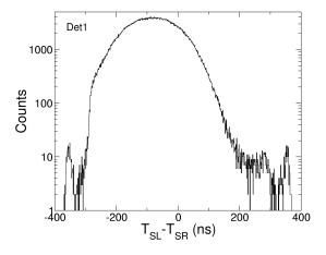
FIGURE 4.22: Spectrum of time difference  $T_{SL} - T_{SR}$  (horizontal localization) on detector 1 for fission coming from the <sup>235</sup>U target.
