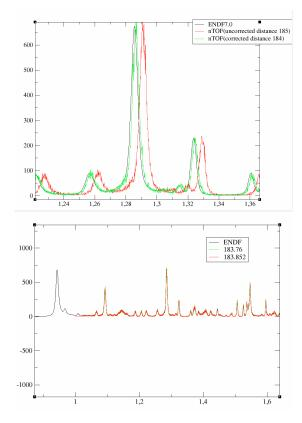
FIGURE 4.6: Comparison of resonant fission cross section of  $^{235}$ U with ENDF/B-VII.0. Upper diagram: a first gess of  $L_{geom}$  has been used. Lower diagram:  $L_{geom}$  has been tuned to match the ENDF/B-VII.0 cross section.
