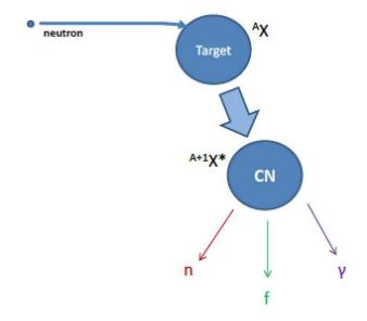
Figure 2.6: Neutron-induced reaction leading to compound-nucleus  $^{A+1}X^*$  [3]
