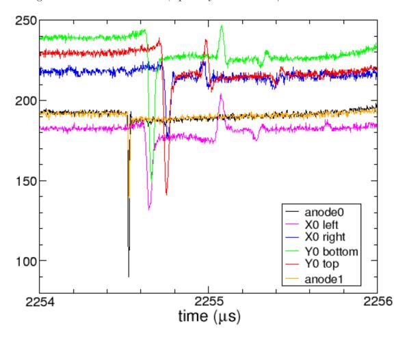
FIGURE 4.2: Expanded view around a fission event of the 5 frames recorded on detector 0 and the anode of detector 1, surrounding the <sup>235</sup>U target. The anode peaks coincide in time showing a coincidence of the fission fragments. The X0 and Y0 peaks are delayed due to the propagation in the delay line. The afterpulses in X0 and Y0 frames are reflections in the delay line due to a mismatch of the impedance of the delay line and the pre-amplifier.
