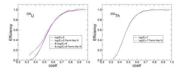
FIGURE 5.15: Comparison of the efficiency with its fit with a fermi-like functional according to 5.18 for  $^{235}$ U (left part) and  $^{232}$ Th (right part).
