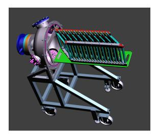
FIGURE 3.12: Ensemble of 10 detectors and 9 targets tilted by 45° against the neutron beam. The holding craddle is fastened on the closing dome mounted on a chariot for transportation.
