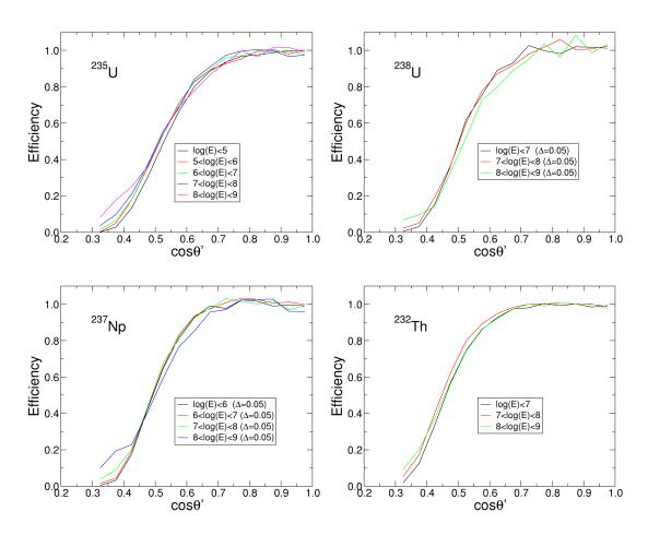
FIGURE 5.14: Detection efficiency as a function of  $\cos \theta'$  for <sup>235</sup>U (top-left), <sup>238</sup>U (top-right), <sup>237</sup>Np (bottom-left), <sup>232</sup>Th (bottom-right) for different energy intervals. Horizontal slices of height  $\Delta \cos \theta' = 0.05$  have been used, and the labels refer to energy intervals defined with their limits in log (E eV).
