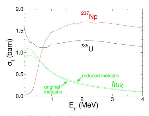
Figure 7.6: Effect of a distortion of the inelastic cross section on the neutron flux and fission cross sections of  $^{237}{\rm Np}$  and  $^{235}{\rm U}$ .
