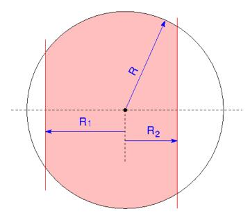
FIGURE 5.13: For a given emission direction  $(\cos \theta', \phi')$  limitation of the possible emission points on the target due to to limited detection area of the detectors.
