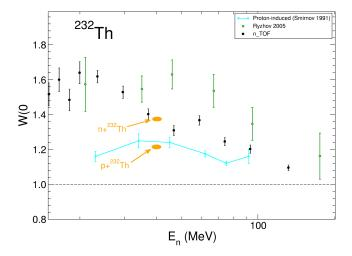
FIGURE 6.7: <sup>232</sup>Th anisotropy with Ryzhov data, n\_TOF data and proton-induced data from Smirnov [6].
