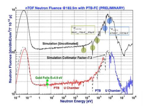
FIGURE 3.3: Phase I n\_TOF neutron fluence simulated and compared to measurements behind a 1.1 cm collimator.
