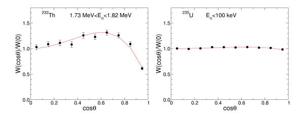
FIGURE 5.17: Left: angular distribution for  $^{232}$ Th for a narrow energy interval about the 1.6 MeV resonance where fission is sideward peaked. Right: same for  $^{235}$ U at low energy where the emission is isotropic, represented with the same scale. The points represent the data with the statistical error bars whereas the red curve is the Legendre polynomial fit with  $P_2$  and  $P_4$ .
