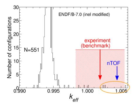
FIGURE 7.7: Spectrum of  $k_{eff}$  for the <sup>237</sup>Np benchmark computed with acceptable random variations of the inelastic cross section of <sup>235</sup>U. The red arrow indicates the benchmark value and the red hatched area the associated uncertainty.
