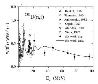
FIGURE 6.9: <sup>238</sup>U anisotropy calculated with SSPSM by Ryzhov.
