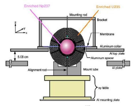
Figure 7.2: Overall scheme of the composite ( $^{237}$ Np and HEU) assembly in compact configuration.
