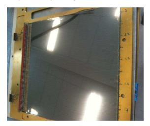
FIGURE 3.7: Stripped cathode of PPAC
