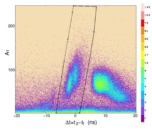
FIGURE 4.8: Correlation between amplitude on detector 1 with the time difference between detectors 2 and 1. The  $^{238}$ U is between detectors 1 and 2, the  $^{235}$ U target is upstream and a  $^{232}$ Th is downstream.
