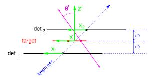
FIGURE 4.24: Top view of the 2 PPACs surrounding the emitting target. The X coordinate is defined in each plane by the green arrows the 0 is the geometric center of the detectors and the target. The Y axis points out upward from the plane and is common to the 2 detectors and the target.
