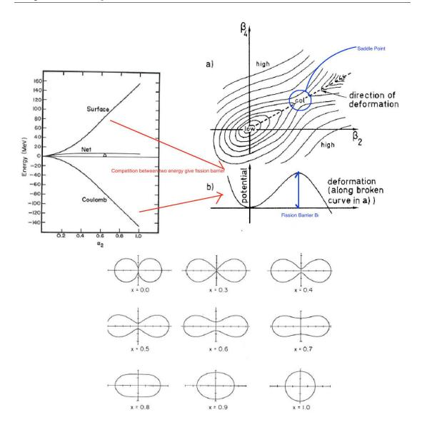
FIGURE 2.2: The fission barrier is a deformation energy of nucleus resulting from the competition between surface energy and Coulomb energy. Illustration with deformation described with quadrupolar and hexadecapolar terms [2].
