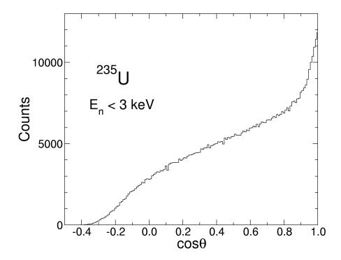
Figure 5.4:  $\cos \theta$  spectrum for <sup>235</sup>U and  $E_n < 3$  keV, proportional to the detection efficiency
