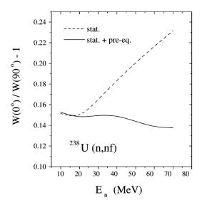
FIGURE 6.2: <sup>238</sup>U anisotropy calculations with and without the inclusion of a pre-equilibrium model [5].
