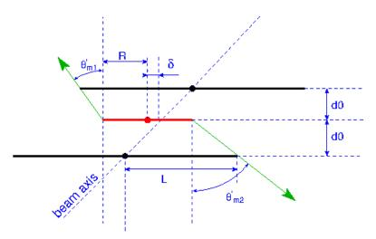
FIGURE 5.12: Top view of 2 detectors and target showing that at smal  $\cos \theta'$  trajectories emitted from the edge of the target may fall outside the active area.  $\delta$  is the horizontal shift of the target, R its radius, L the half length of the active area and  $d_0$  the separation distance.
