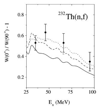
FIGURE 6.3: Comparison of  $^{232}$ Th FFAD (points) and SSPSM model (solid line) and within the effect of 30% reduction of  $K_0^2$  (dashed line), from [5].
