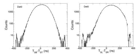
FIGURE 4.21: Spectra of time differences  $T_{SB} - T_{ST}$  (left) and  $T_{SL} - T_{SR}$  (right) representing the Y and X localization in detector 0 of figure 4.9.
