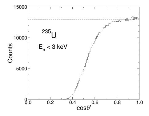
FIGURE 5.1: Distribution of  $\cos\theta'$  for  $^{235}\mathrm{U}$  and  $E_n < 3$  keV. As the emission is isotropic a full efficiency would lead to a constant number of counts as depicted by the horizontal dashed line.
