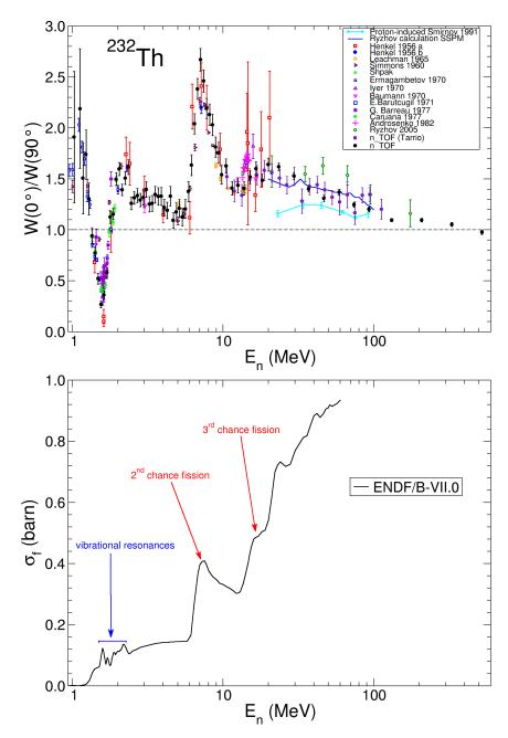
FIGURE 6.1: Upper part:  $^{232}$ Th anisotropy, the n\_TOF data are the black points and previous measurements. The lower part represents the  $^{232}$ Th fission cross section and the successive fission chance openings.
