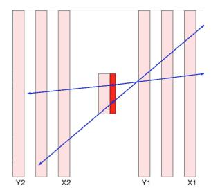
FIGURE 3.9: Fission fragment lost due to the stopping of the fission fragment at large angle
