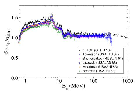
Figure 7.1: Comparison of different  $^{237}$ Np fission cross sections measured relative to  $^{235}$ U.
