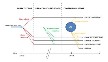
Figure 2.5: Conceptual view of a nuclear reaction
