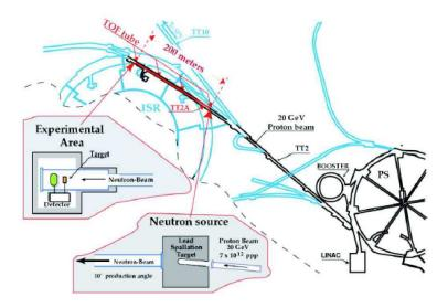
FIGURE 3.1: Sketch of the n\_TOF facility at CERN with expanded views of the spallation target area and the experimental area
