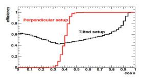
Figure 3.11: Simulation of detection efficiency for the 2 geometrical configurations: orthogonal to the beam and tilted by 45° [4]
