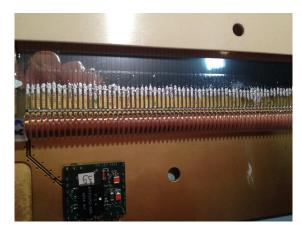
FIGURE 3.8: Expanded view of the cathode frame showing the delay line, the capacitors between strips, the connections with silver pastry, the charge preamplifier.
