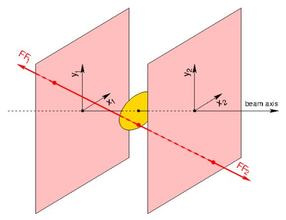
Figure 3.6: Principle of measurement of the fission angle with 2 PPACs
