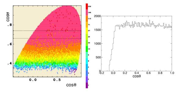
FIGURE 5.10: Left: distribution of counts divided by the solid angle for the  $^{235}$ U target and  $E_n < 100$  keV. Right: projection on  $\cos \theta$  of the band of constant efficiency (constant  $\cos \theta'$ ), drawn on the left size.
