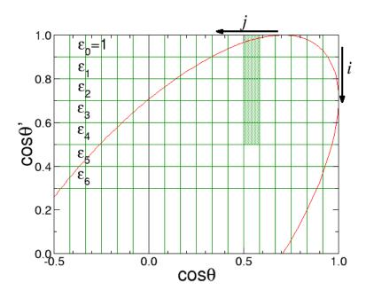
FIGURE 5.11: Partitioning of the  $(\cos \theta, \cos \theta')$  plane into a matrix of cells. Along horizontal lines the cells have the same efficiency. The columns correspond to the  $\cos \theta'$  values where the angular distribution has to be obtained. The lines are numbered with i, starting from the top, and the columns are numbered with j starting from the right.
