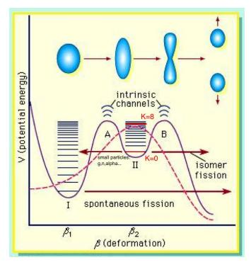
FIGURE 2.4: The double-humped fission barrier.
