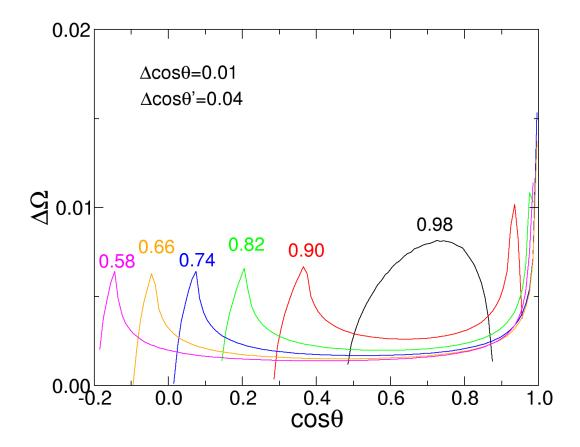
FIGURE 5.9: Solid angle of  $(\cos \theta, \cos \theta')$  cells for cells of width  $\Delta \cos \theta = 0.01$  and height  $\Delta \cos \theta' = 0.04$ . The numbers over the curves label the central value of  $\cos \theta'$  of the horizontal band.
