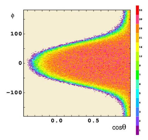
Figure 5.2: Distribution in angles  $(\cos \theta, \phi)$  of isotropic events emitted by the  $^{235}\mathrm{U}$  target for neutron energies  $E_n < 3$  keV.
