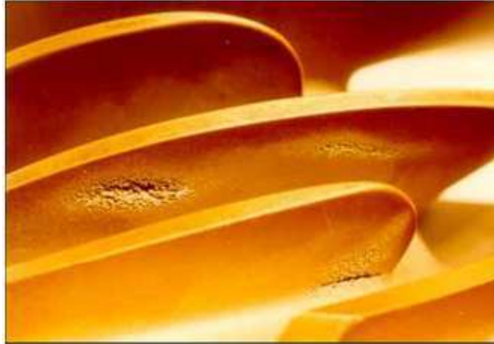
Figure 1.2: Image of typical cavitation damage on the blade of a mixed flow pump [9]
