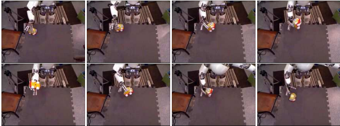
FIGURE 8.7 – Examples of images, where an object is explored based on TakeObserve manipulation : the object is grasped, lifted, rotated, approached at a closer distance, turned around to observe its different perspectives, and posed back to the table
