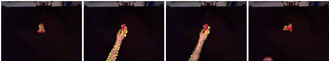
FIGURE 4.7 – Examples of extracted and tracked GFT points in the sequence of four images : all extracted points are shown by big yellow circles, and tracked points are marked by small black circles inside yellow circles
