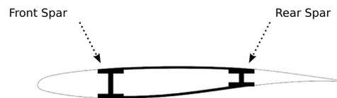
**Figure 4.3:** Primary structure elements in a wing cross section
