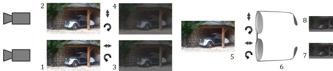
Figure 3.5: The functioning of a polarization stereoscopic system; adapted from [Sony 3D Television & Film 2010].
