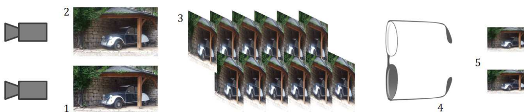
Figure 3.6: The functioning of a stereoscopic system using shutter glasses; adapted from [Sony 3D Television & Film 2010].
