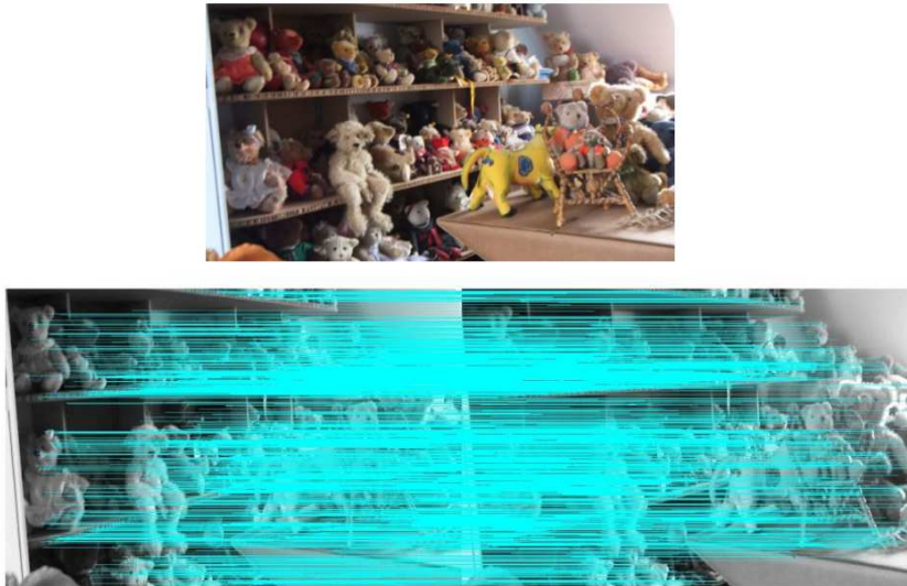
Figure E.2: Example of a stereo-match determined with our algorithm based on the SIFT feature detection method.
