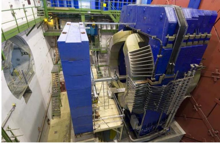
Figure 5.3: View of the muon filter (left) and of the dipole magnet (right).
