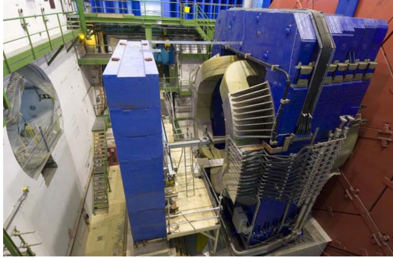
Figure 5.3: View of the muon filter (left) and of the dipole magnet (right).
