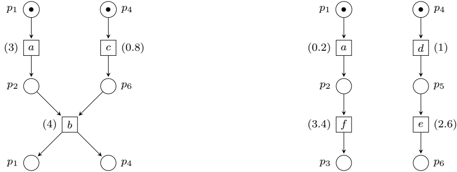
Figure 2.3: Two processes of the time Petri net of Figure 2.2. The occurrence dates are written in parentheses near the events.
