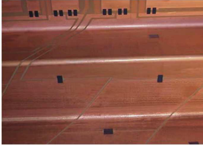
FIGURE 3.11: Pair of high-voltage distribution resistors (upper) connecting the HV bus to the back sampling or directly to the middle cells by narrow copper traces. Both pictures are from a bent B electrode but representative of all other types [82].
