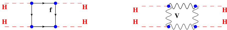
FIGURE 1.5: Diagrams for the one-loop contributions of fermions and gauge bosons to \lambda .
