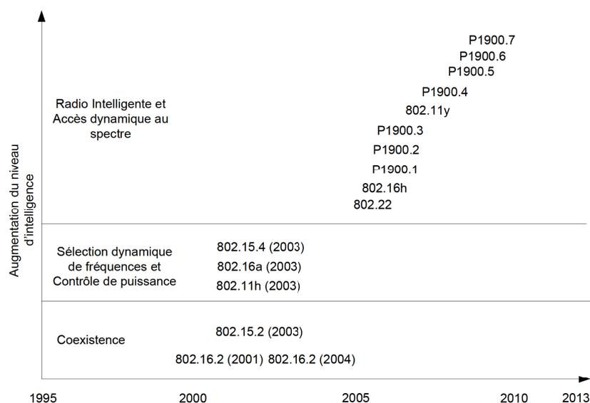
FIGURE A.1 – Classification des standards de la radio intelligente [11]
