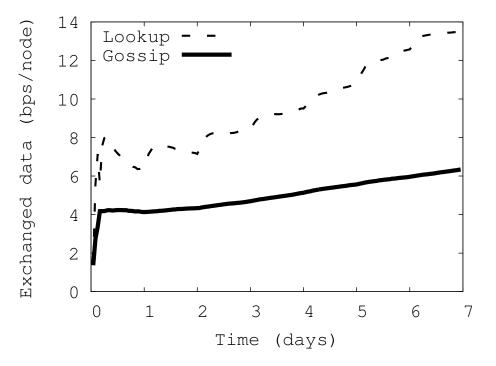
Figure 6.11: Evolution of the network load with the Overnet trace.
