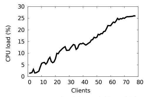
Figure 7.2: Server CPU load. 100% of CPU load accounts for full usage of the four cores. The Quake III server uses one core only.
