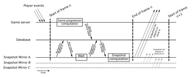
Figure 7.5: Exchanges during frame computation (for clarity, only the queries of Snapshot mirror A *are represented*)
