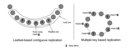
Figure 9.1: Leafset-based and multiple-key-based replication (k = 5).
