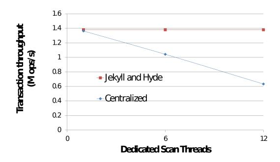
Figure 10.2: Transactional throughput as a function of scan threads.
