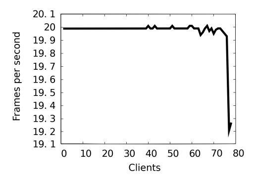
Figure 7.3: Server frames per second. Rates below 20 fps degrade gaming experience.
