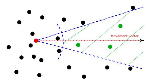
Figure 5.1: Blue Banana prefetches peers inside the cone centered on the trajectory, except peers that are too close to be contacted on time.
