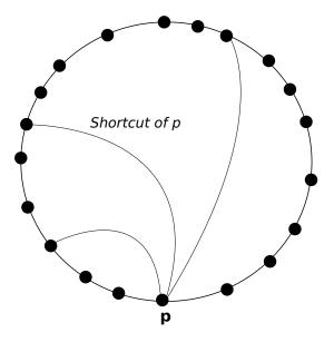
Figure 2.3: Ring topology augmented with shortcut-links (only shortcuts of the peer p are represented).
