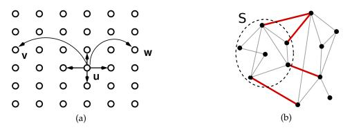
Figure 2.4: (a) Kleinberg model: 2D lattice with shortcuts, (b) Expansion: Bold edges represent  $\delta S$
