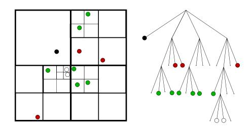
Figure 3.3: Subdivision resulting from a non uniform peer-distribution and the corresponding quadtree structure.
