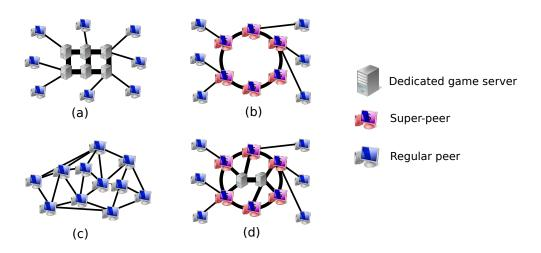
Figure 3.2: *Main topologies for NVEs: (a) pure c/s; (b) multi-tier p2p; (c) nearest-neighbor p2p; (d) hybrid.*
