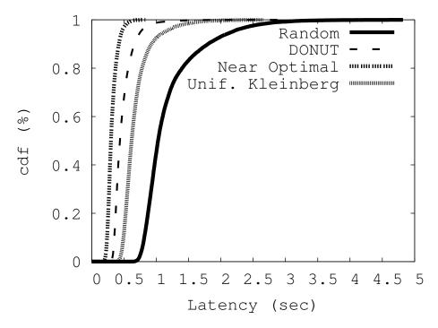
Figure 6.12: *Cumulative distribution function (cdf) of mean routing latencies for an overlay of* 2500 *nodes.*
