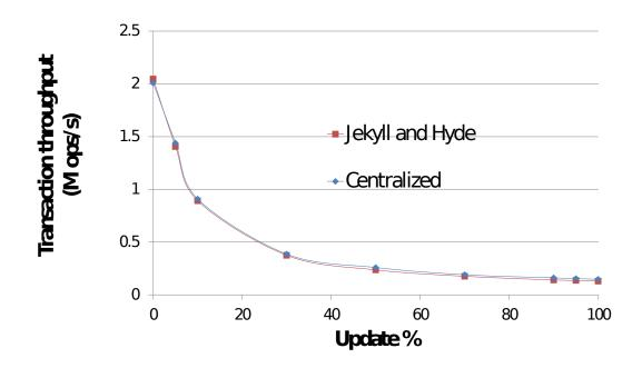
Figure 10.5: Overall transaction throughput as a function of update ratio.
