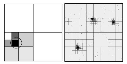
Figure 6.3: *Left: After local execution of Algorithm 2 on a void map. (the greyscale represents the density, black being the highest). Right: Approximation of a keyspace with three density zones.*
