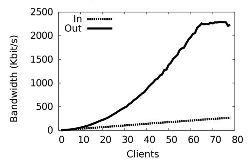
Figure 7.1: Server bandwidth consumption. Incoming: linear, Outgoing: supra-linear growth.
