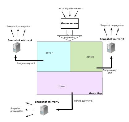
Figure 7.4: The load of snapshot propagation is shared through NVE partitioning.
