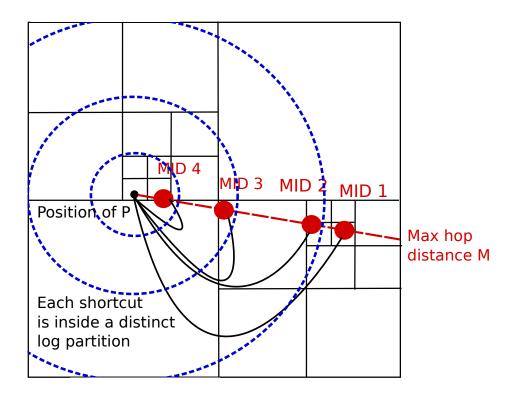
Figure 6.5: Execution of the log-partition algorithm on the local map of the peer P.
