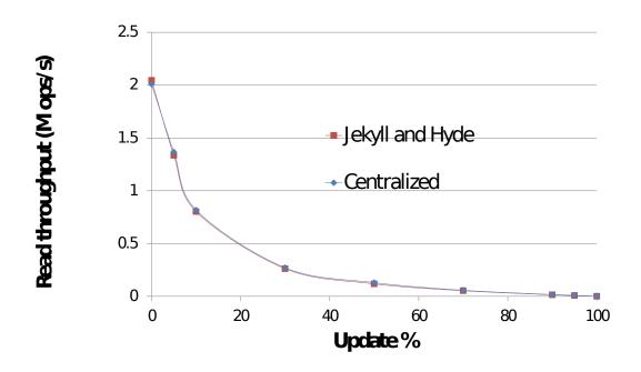
Figure 10.6: Read transaction throughput as a function of update ratio.
