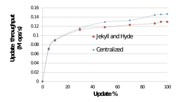
Figure 10.7: Write transaction throughput as a function of update ratio.
