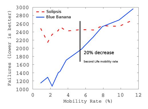
Figure 5.3: Average number of overlay transient failures per second (lower is better).
