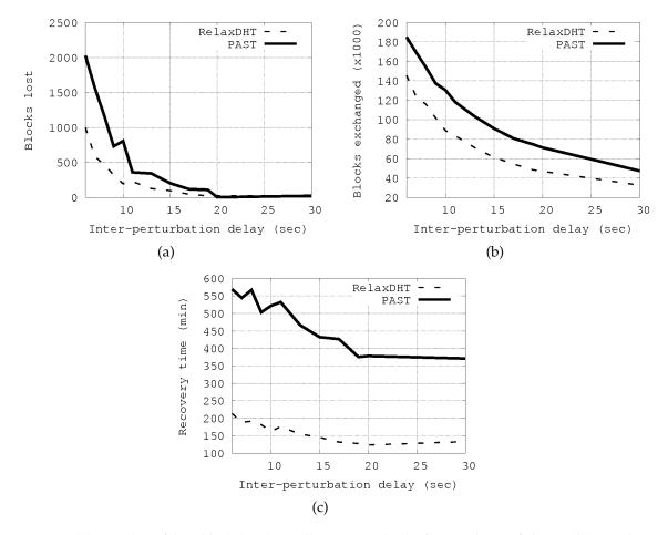
Figure 9.4: (a) Number of data block lost (i.e., all copies are lost) after one hour of churn, (b) Number of exchanged data blocks to restore a stable state after one hour of churn, (c) Recovery time: time for retrieving all the copies of every remaining data block.
