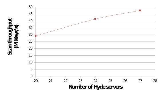
Figure 10.8: Scan throughput versus number of Hyde servers.
