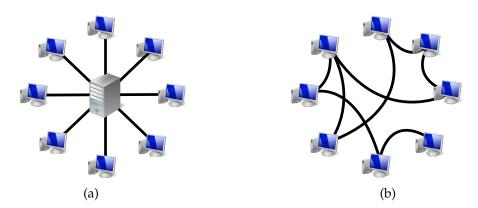
Figure 2.1: (a) Client-server topology, (b) Example of peer-to-peer topology
