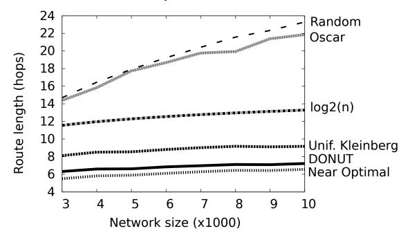
Figure 6.6: Scalability test: Mean route length in function of the overlay size.
