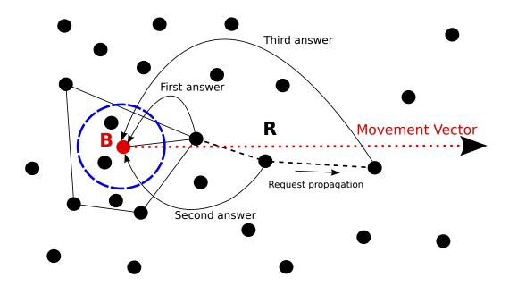
Figure 5.2: Propagation algorithm: the request is transmitted to peers ahead of the movement.
