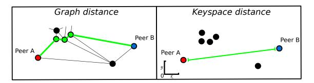
Figure 6.4: *Graph distance in number of hops vs Keyspace distance (euclidean distance) between peers A and B.*
