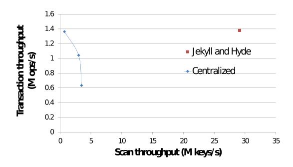
Figure 10.4: Tradeoff between scan and transactional throughput.
