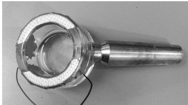
FIGURE 4.2 – Transparent mouthpiece developed by Castellango et al. [CCS83] equipped with copper foil shielding tape electrodes.
