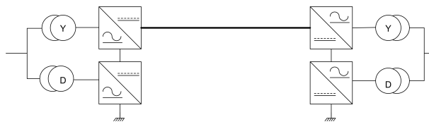
Figure 1.3: +U monopolar link scheme with ground return
