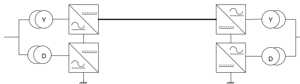
Figure 1.3: +U monopolar link scheme with ground return
