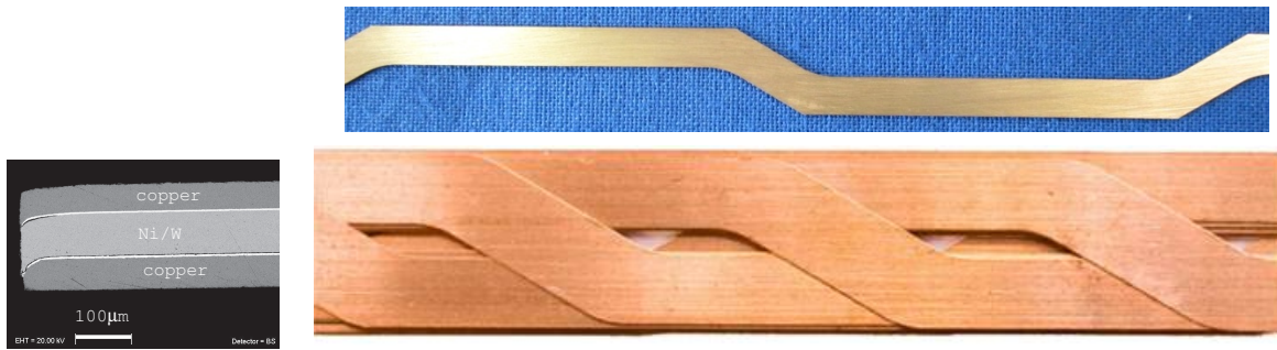
Figure 2.14: Cross section of a punched YBCO conductor [73] (left). At the right: top view of a meander YBCO tape conductor with a 126 mm transposition pitch (top). Top view of a 15 strand YBCO Roebel cable with a transposition pitch of 300 mm [81] (bottom).
