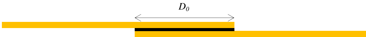
Figure 3.28: Longitudinal schematic view of a lap joint. The two conductor are soldered over an interfacing distance D_0 .
