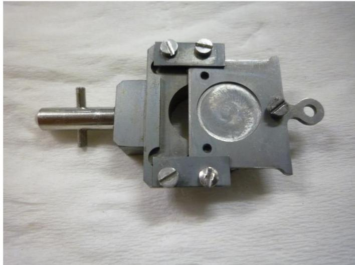
*Fig. 2.8. Photograph of the realized detachable sample holder.*
