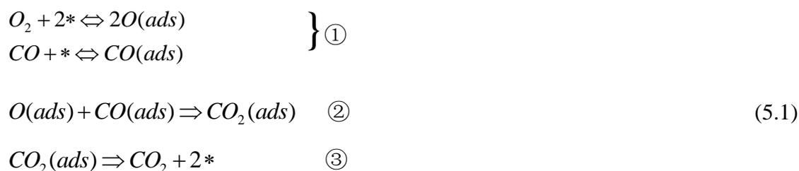
where \* represents an empty site. The first step is O<sub>2</sub> adsorption and dissociation and CO adsorption; the second is O(ads)+CO(ads) reaction to CO<sub>2</sub>; the third is CO<sub>2</sub> desorption. O<sub>2</sub>
