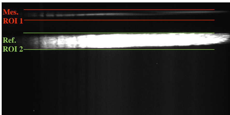
Fig. 1.12. Display of the two SFG signals on the detector: sample and reference at two ROI of the CCD.
