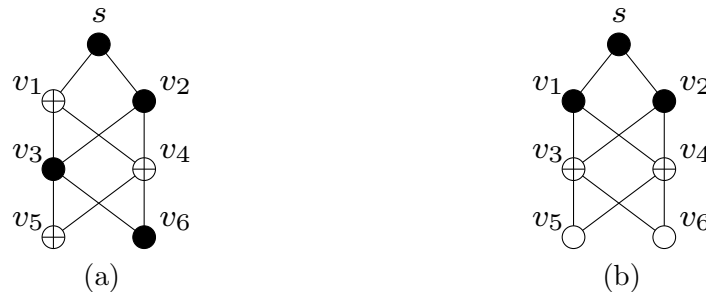
Figure 5.3: In the figure (a) the applied strategy consists of protecting a vertex adjacent to the fire at each step. The strategy of figure (b) protects vertex v_3 at time step one and v_4 at time step two. The later strategy save one more vertex than the former one. The burned vertices are represented by black vertices. A protected vertex is represented by a circle with a cross inside.
