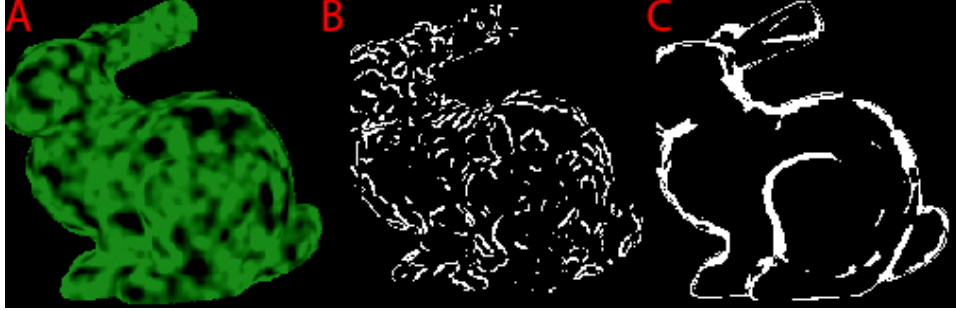
Figure 5.2: A. Stanford bunny image. B. The best 15% pixels selected by image gradients. C. The best 15% pixels selected by depth gradients. Combination selection is required for constraining the motion the most efficiently.
