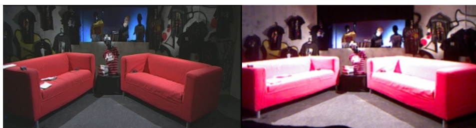
Figure 8.6: HD camera (left) and Microsoft Kinect RGB image (right) in a typical studio lighting conditions.
