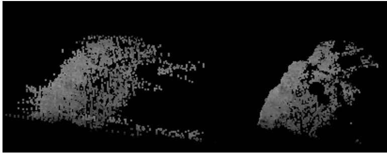
Figure 4.10: The difference in rock reconstruction quality between multi-resolution SAD (on left) and SGBM (on right). The rock image is illustrated in Fig. 4.9.
