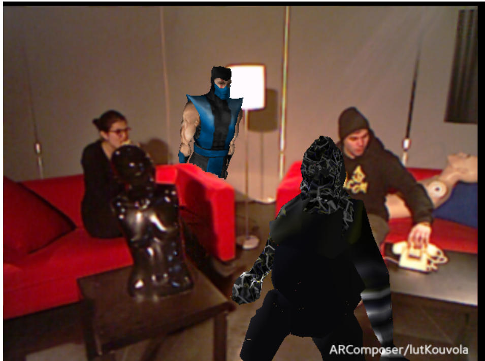
Figure 8.4: A real-time AR broadcast with virtual 3D characters which are rendered from the estimated pose using Panda3D. See example video 1 .
