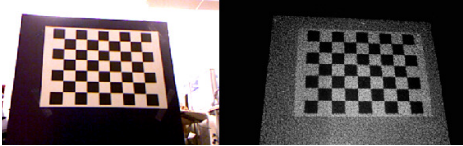
Figure 2.10: RGB and IR images of the calibration pattern.
