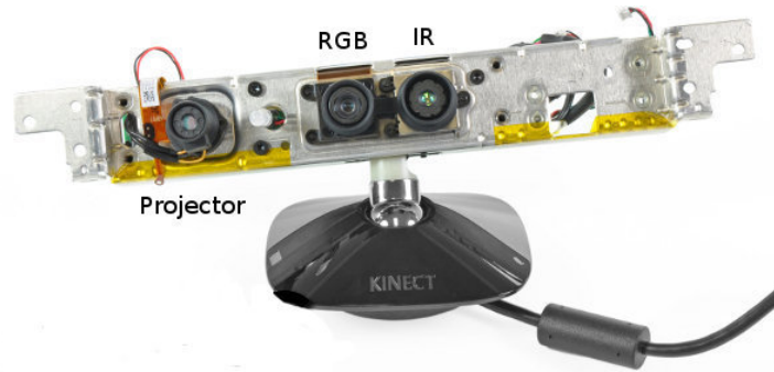
Figure 2.9: Microsoft Kinect the plastic cover removed. Image is courtesy of www.ros.org .
