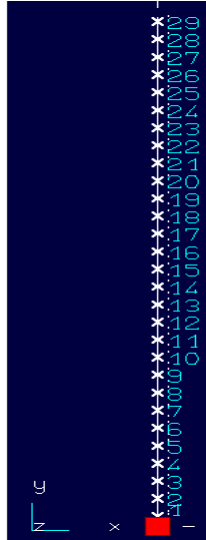
Figure III. 1: Clamped-free beam model in 1D with modal analysis using FEM by RDM6.
