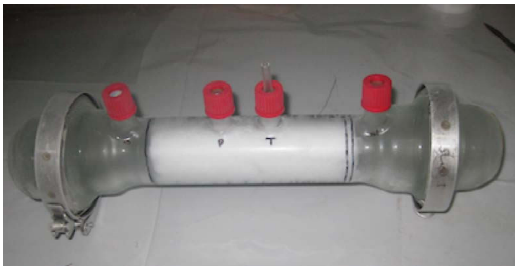
Figure 3.2. Photo of the glass cell filled with a snow within the teflon sleeve and the four ports
