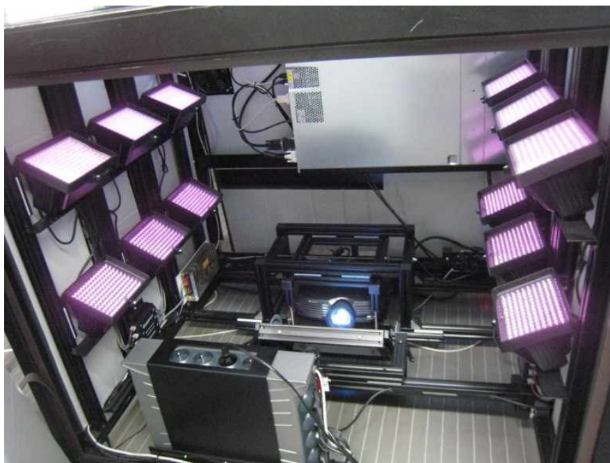
Figure III.6: Inside of the ILight Table: infrared rays are projected onto the touch surface by ranges of diodes located below it. An infrared camera located below the surface transmits the video stream to a computer which determines the position with image processing algorithms
