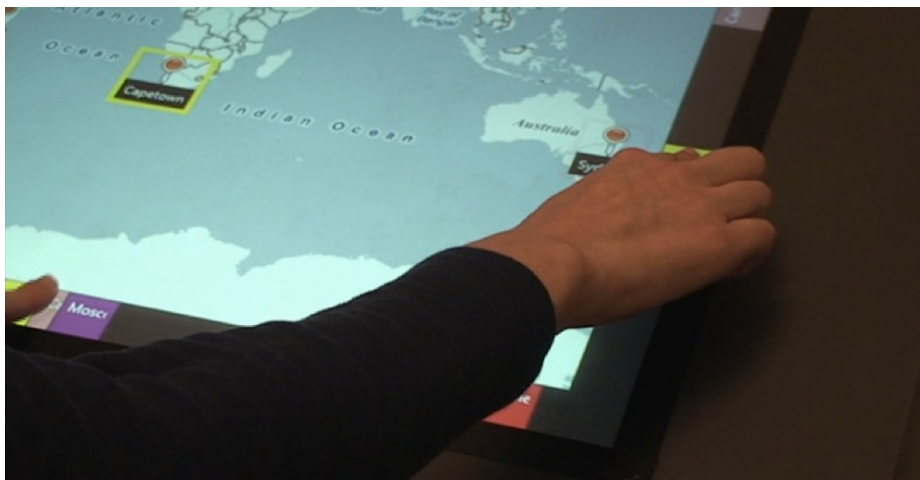
Figure II.17: Access Overlays as presented by (Kane, Morris, et al., 2011). The image shows the edge projection technique. The user is exploring the menu on the x- and y-axis. Reprinted with permission.
