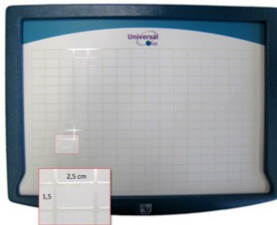
Figure III.3: Geotact tablet by E.O. Guidage. This device offered a 16*16 matrix of rectangular interactive zones, thus providing 256 touchable zones. Reprinted from (Brock, Molas, et al., 2010).
