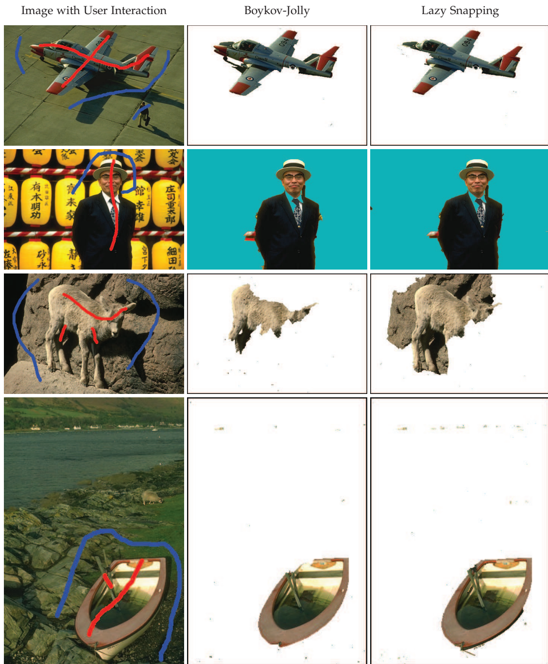
Figure 2.7: Segmentations results by Boykov-Jolly method [23] and Lazy Snapping [65] on natural color images from Berkeley Segmentation Dataset [35]. First column: original color images include "Plane" (Ref. 37073), "Japanese" (Ref. 65019), "Sheep" (Ref. 41025) and "Boat" (Ref. 92059). Second column: segmentations obtained by Boykov-Jolly method. Last column: segmentations obtained by Lazy Snapping .
