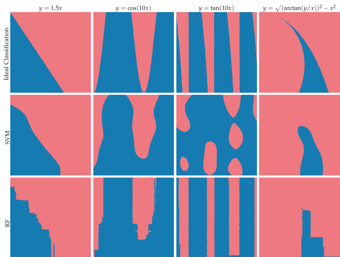
Figure 3.9: Comparison of SVM and RF on synthetic datasets.
