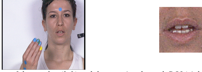
Figure 4.1: Image of the speaker (left) and the associated mouth ROI (right). The landmark in the center of the speaker's eyebrows is used to locate the mouth ROI.
