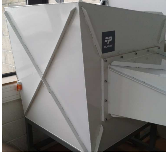
FIGURE B.3 – Caisse de tranquillisation.
