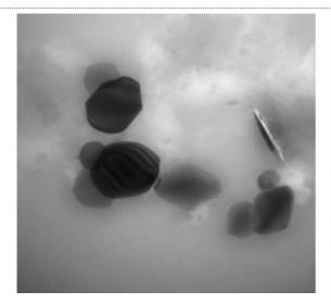
**Figure 70:** TEM imaging of NS entry 25, magnifying x100,000.
