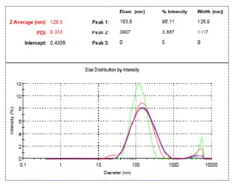
Figure 93: Particle Size distribution of entry 1 Table 29.
