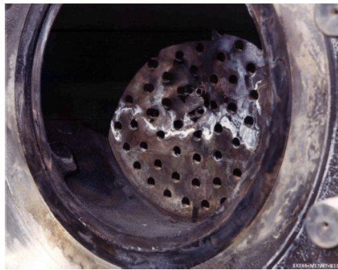
Figure 1.9: Damaged rocket chamber from combustion instabilities.
