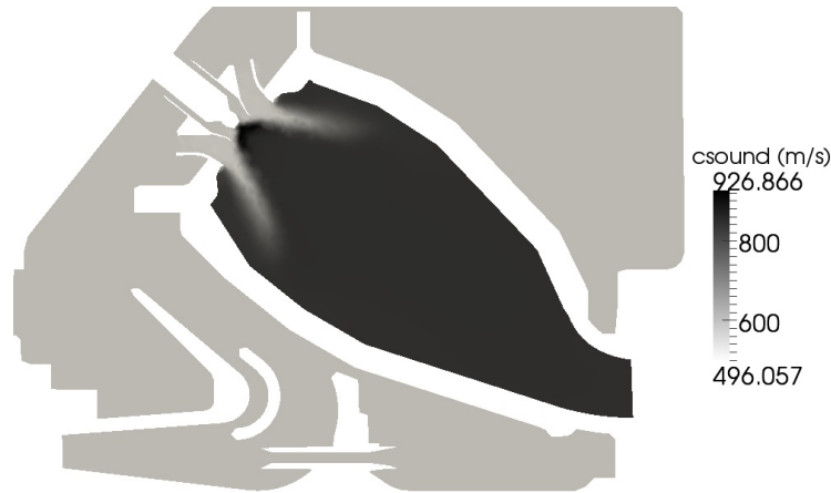
Figure 6.4: Longitudinal cut: sound speed c_0(\vec{x}) field obtained from a LES time-average solution used for AVSP simulations.
