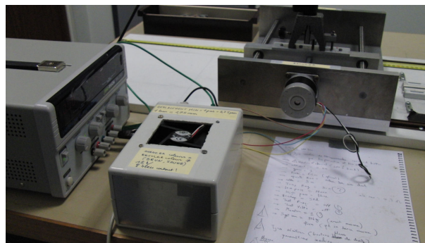
Figure E.7: Illustration of the home-made one-dimensional positioning system used to measure transverse and longitudinal velocity profiles.
