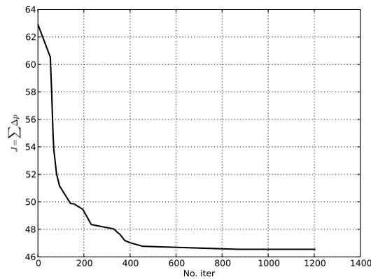
Figure 5.26: Objective function ( $\sum \Delta p$ ) for the wing optimization adopting a shaped nose fuselage.
