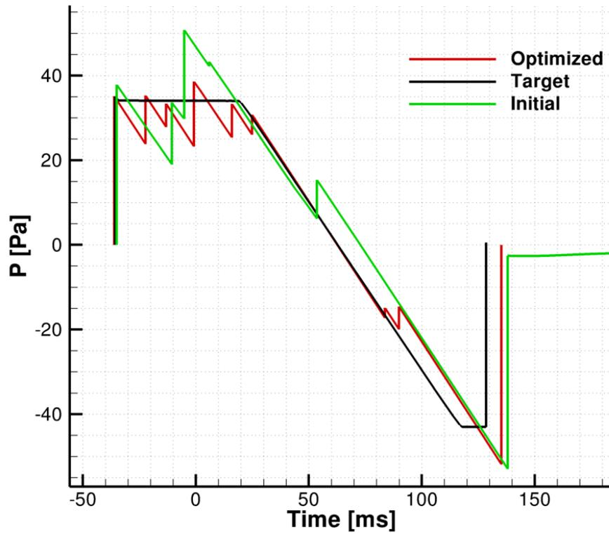
Figure B.26: Comparison of the obtained ground signature.
