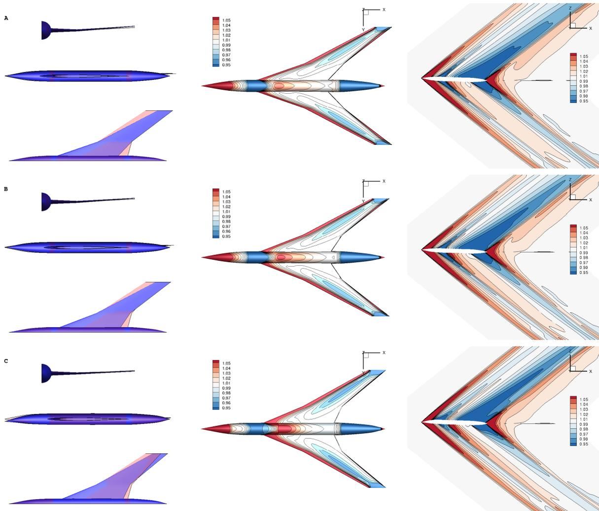
Figure 6.21: Geometry configuration, bottom skin pressure ( $p/p_0$ ) and symmetry plane pressure ( $p/p_0$ ) in near field for configuration A, B and C on the Pareto front (In red the initial geometry).
