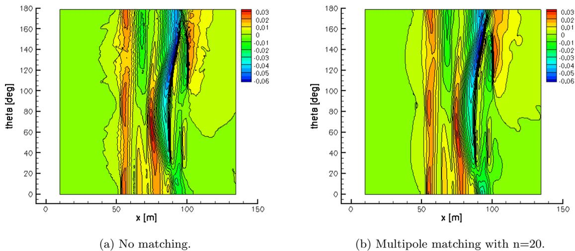
Figure B.11: Pressure  $((p - p_\infty)/p_\infty)$  extrapolated over a cylinder ( $R/L=1$ ).
