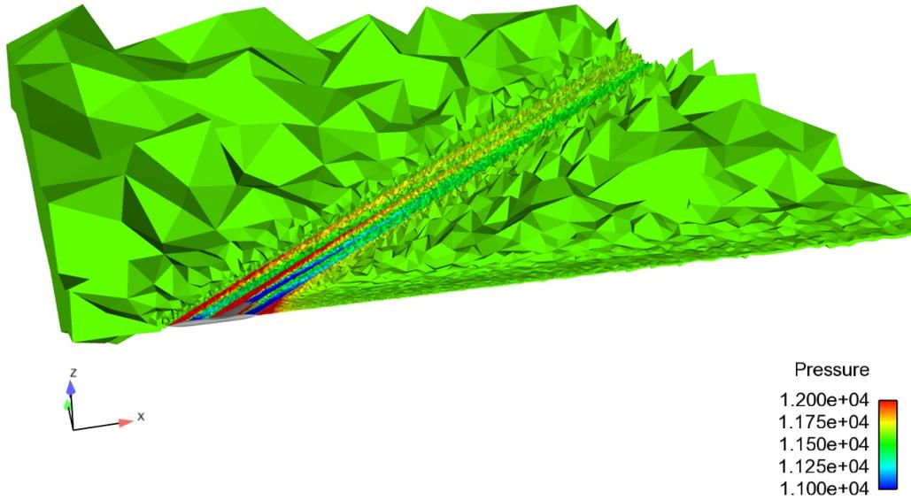
Figure 3.29: Crinkly plane showing pressure distribution in the plane  $z = 0$ . 20<sup>th</sup> adaptation.
