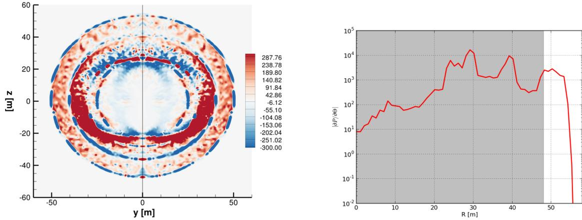
Figure 3.31: Azimuthal pressure gradient and  $\max_{\theta} \left| \frac{\partial P}{\partial \theta} \right|$  in the near-field ( $x = 3L$  after the nose top). In gray the estimated position of the front shock.
