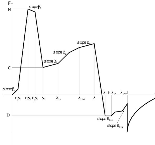
Figure 4.5: Generalized F-function for front and aft shaping.
