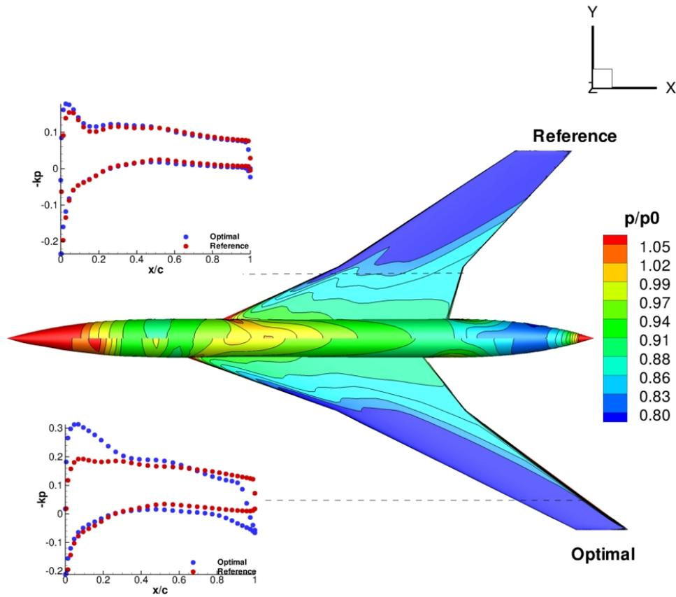
Figure 5.16: Upper skin pressure distribution and pressure coefficient at different wing sections ( $y = 4$  m and  $y = 8$  m).
