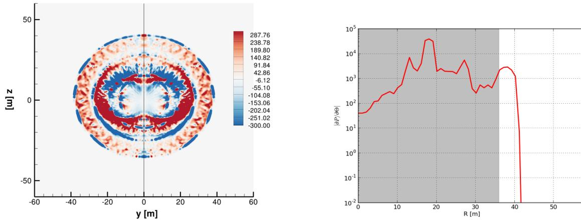
Figure 3.30: Azimuthal pressure gradient and  $\max_{\theta} \left| \frac{\partial P}{\partial \theta} \right|$  in the near-field ( $x = 2L$  after the nose top). In gray the estimated position of the front shock.
