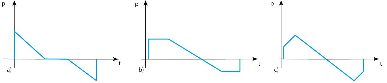
Figure 4.1: Different ground signature that can be obtained using the Jones and Seebass parameterization: a) minimum impulse, b) minimum shock overpressure, c) minimum shock pressure rise.
