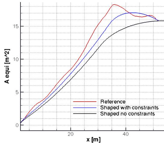
Figure B.17: Equivalent area. Shaped configuration with and w/o volume constraint.
