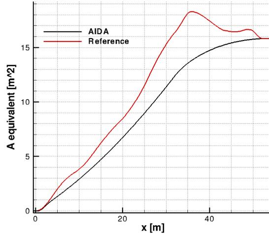
Figure B.14: Equivalent area. AIDA shaped configuration.
