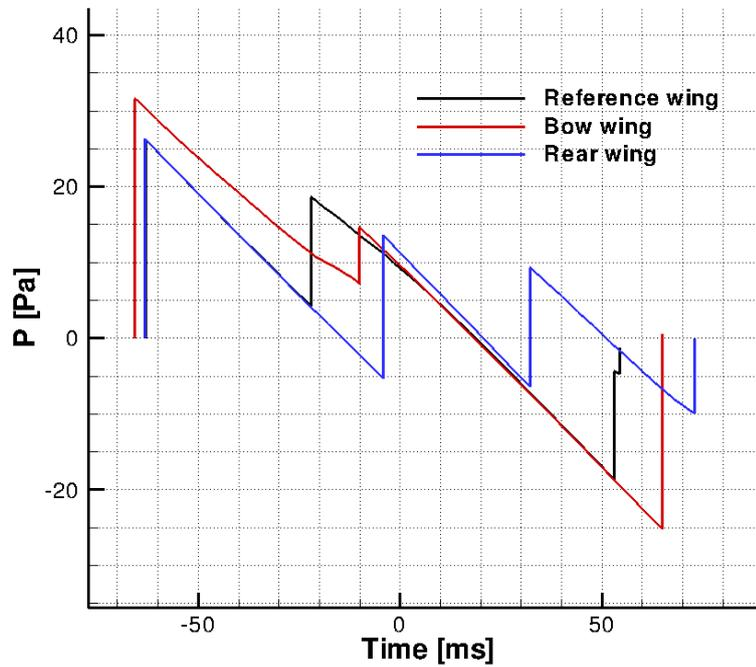
Figure 5.9: Effects of wing position on ground signature.
