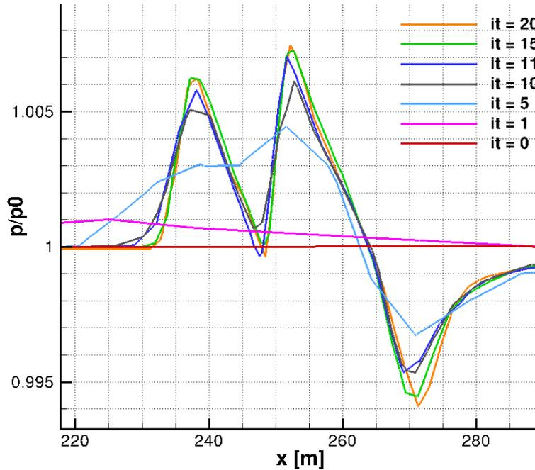
Figure 3.28: Pressure signature at  $R/L = 6$  for different adaptation iterations.
