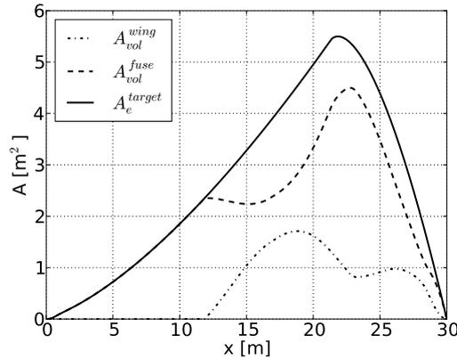
Figure 4.19: Initial tailoring of the fuselage area distribution.
