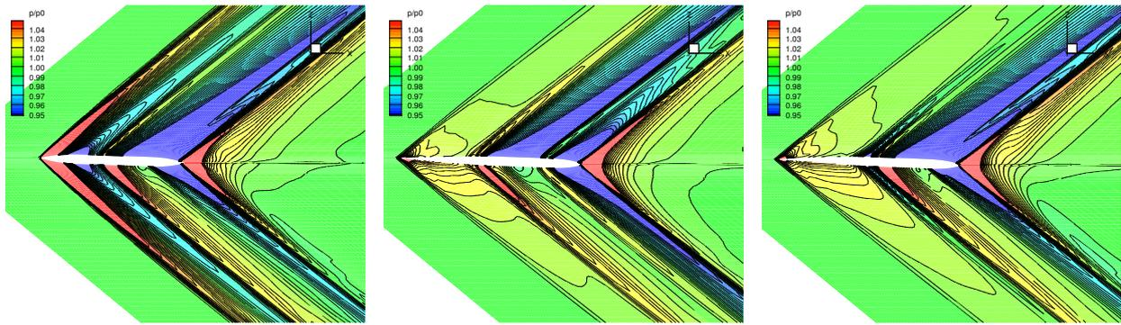
(a) Initial configuration with conventional fuselage. (b) Initial configuration with shaped nose fuselage.
