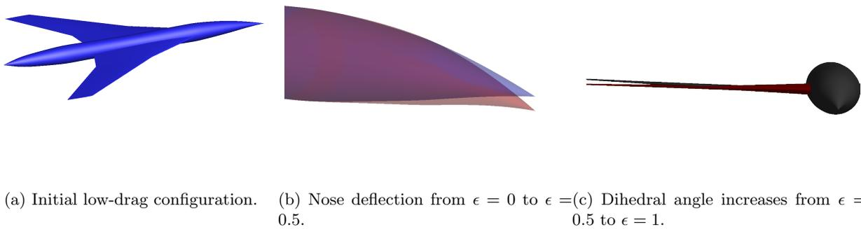
Figure 6.31: Main geometry modifications during Nash game convergence. In blue the initial low-drag configuration ( $\epsilon = 0$ ), in red the configuration at  $\epsilon = 0.5$ , in black the configuration at  $\epsilon = 1$ .
