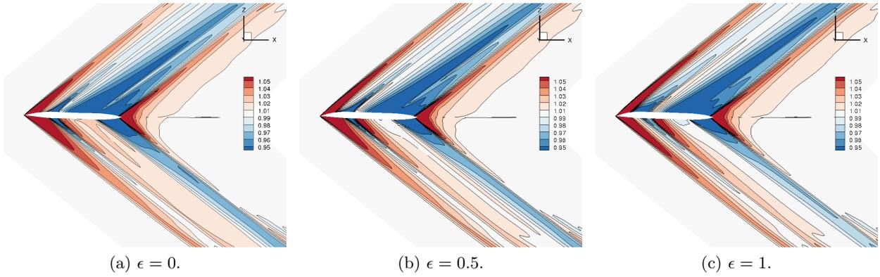
Figure 6.33: Near-field pressure ( $p/p_0$ ) in the symmetry plane.
