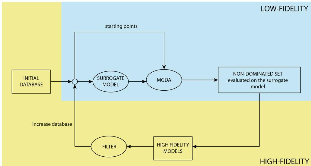
Figure 6.15: MGDA with surrogate model scheme. A surrogate model based on an initial database is trained. Then, MGDA [111] is applied from each database point using surrogate models. Thus a non dominated set on the surrogate model is obtained.
