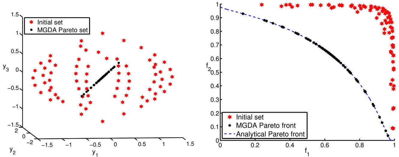
Figure 6.14: Convergence of MGDA from initial design points around Pareto front, for a classical test case proposed by Fonseca, in design space (left), in function space (right).
