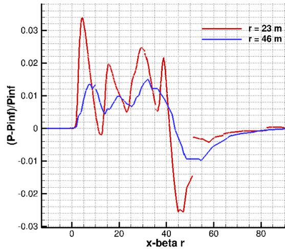
Figure B.7: Under-track pressure perturbation in near-field. Reference configuration.
