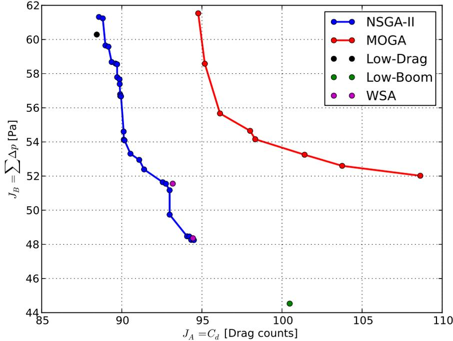
Figure 6.8: Comparison between the Pareto front obtained using NSGA-II, the one obtained using MOGA, the WSA trade-off solutions and the mono-disciplinary optimizations.
