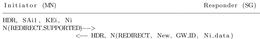
Figure 2.9: REDIRECT support during IKE_SA_INIT
