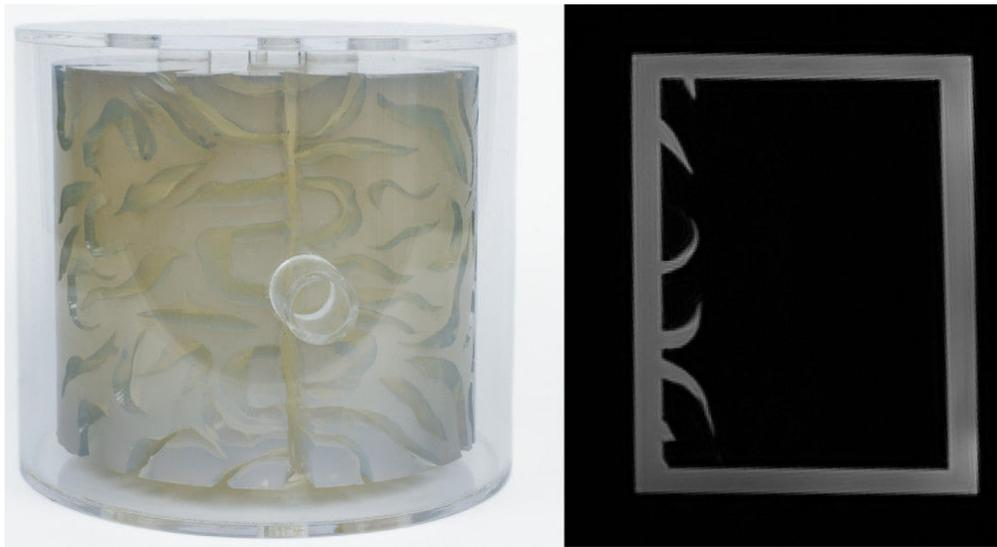
Figure 3.9 – Photography of a synthetic resin phantom (volume:  $1494\text{cm}^3$ ) mimicking the cerebral sulci used to validate the entire cerebrospinal fluid volume segmentation method. Right: cross-section of the corresponding magnetic resonance image.
