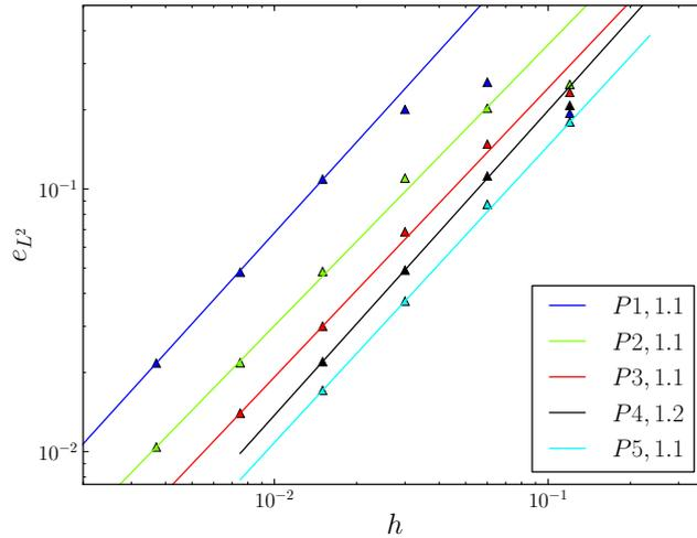
Figure 4.4:  $L^2$  error as a function of mesh size for different polynomial approximation orders ( $\mathbb{P}^n$ ) using a smooth projection method. The legend gives the polynomial approximation order of the initial level set field and the slope associated to the error.
