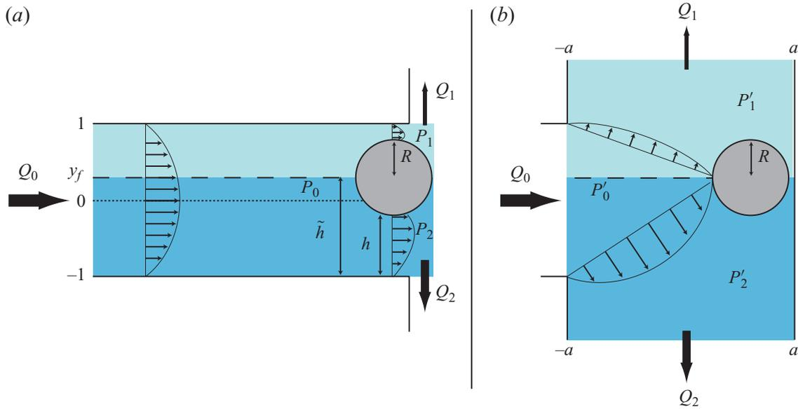
FIGURE 7. (Colour online) Schematic of the geometry considered for the two effects occurring in the bifurcation. (a) Entrance to the bifurcation showing attraction towards the low-flow-rate branch ( $P_1 < P_2$ ). (b) Opposite wall showing attraction towards the high-flow-rate branch ( $P'_1 > P'_2$ ).
