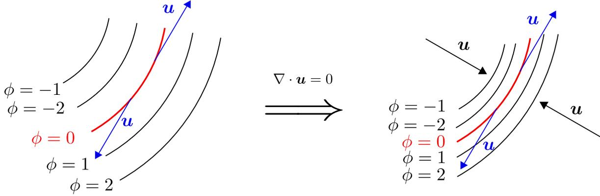
Figure 4.6: Scheme explaining how the divergence free velocity implies that  $|\nabla\phi|$  records the stretching of the interface. If the interface is stretched it means that the velocity field is *pulling* on it from two sides as shown on the left scheme. Since the velocity is divergence free, it has to push in the other direction to fulfill this condition. Thus, the level set lines are getting closer, consequently, the gradient magnitude of  $\phi$  increases.
