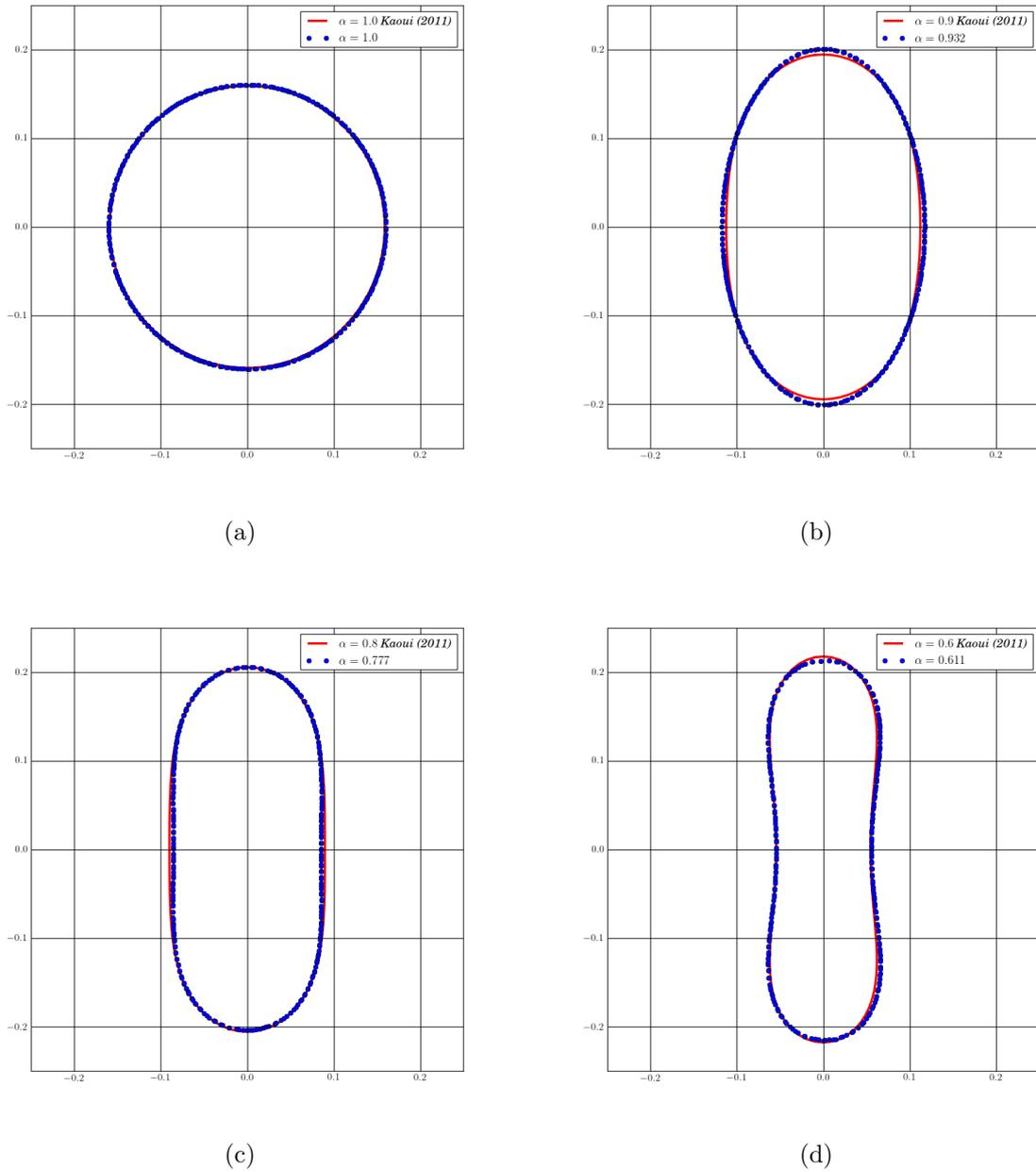
Figure 4.8: Equilibrium shapes of vesicles for different reduced areas. The blue points are our simulations, whereas the red lines are the simulation taken from [53] done by Lattice Boltzmann method. The exact reduced area is given as legend on the graphs. The difference between the two models are mainly due to the change of area in level set method.
