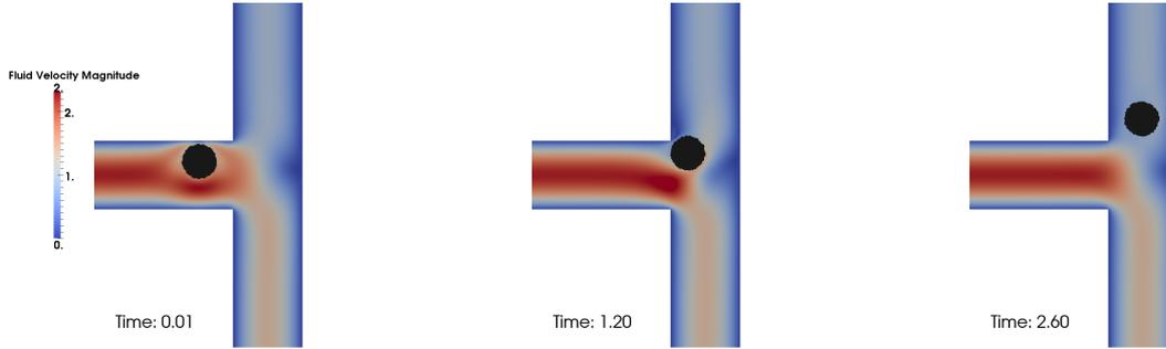
Figure 3.1: 2D simulation of the bifurcation problem presented in section 7.1. The color is the magnitude of the velocity vector  $|\mathbf{u}|$ . The area in which  $\mu = \mu_2$  is represented in black. The particle enters in the low flow rate branch of the bifurcation.
