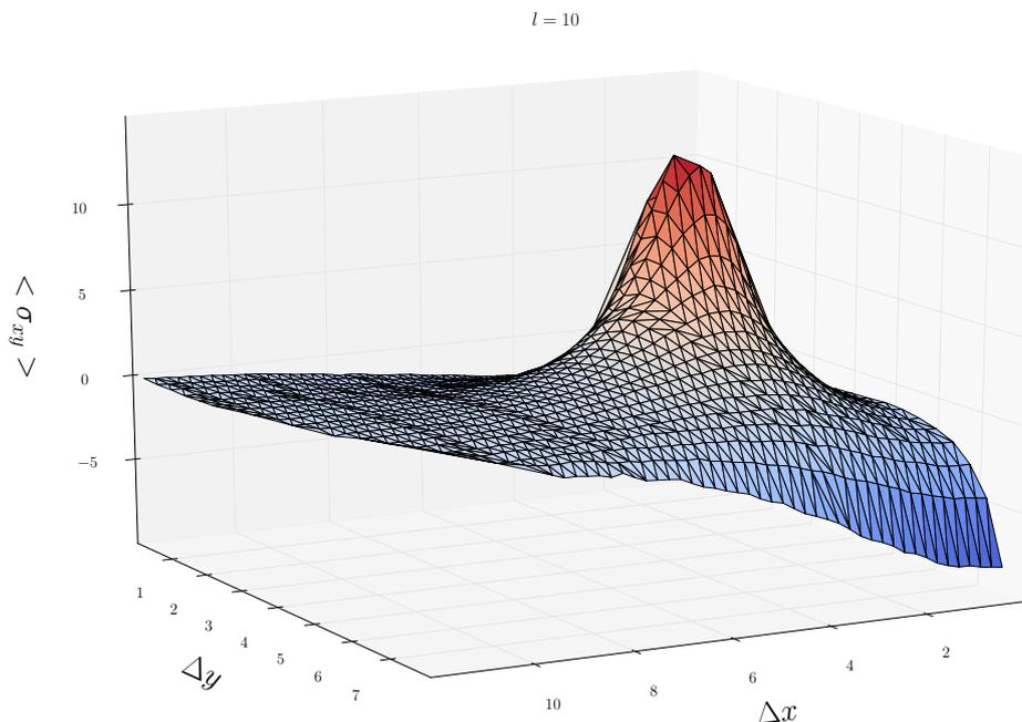
(b) The quantity  $\langle \sigma_{xy}^2 \rangle^{\text{part}}$  represented in elevation. The bottom plane represents the values of  $\Delta x$  and  $\Delta y$ . The color represent the value of  $\langle \sigma_{xy}^2 \rangle^{\text{part}}$ . This quantity has been measured for every point represented on the 3D surface. The lines between the points are just a guide for the eyes.
