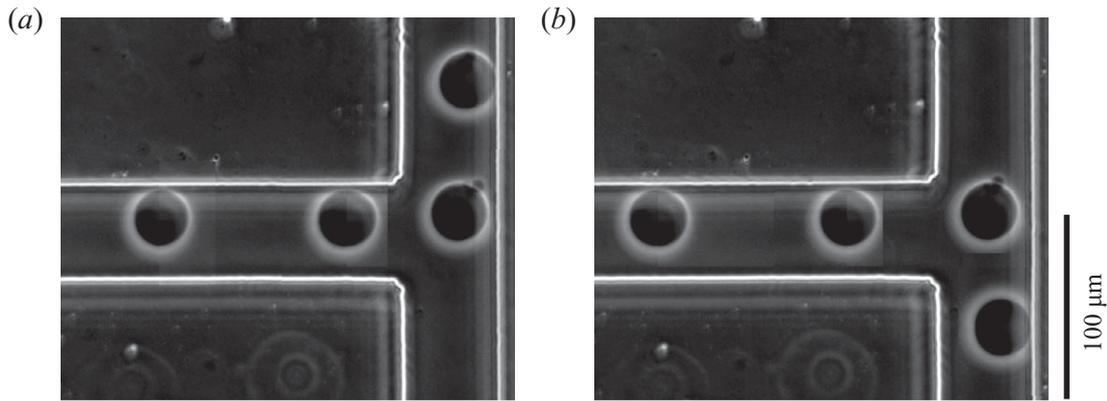
FIGURE 4. Photographs showing the different positions of a vesicle of radius  $R = 0.60$  starting just above and just below its separating line. No clear difference between these two starting positions can be seen by eye, which illustrates the accuracy we get in the measurement of  $y_0^*$ . Here  $Q_1/Q_0$  is set to 0.28.
