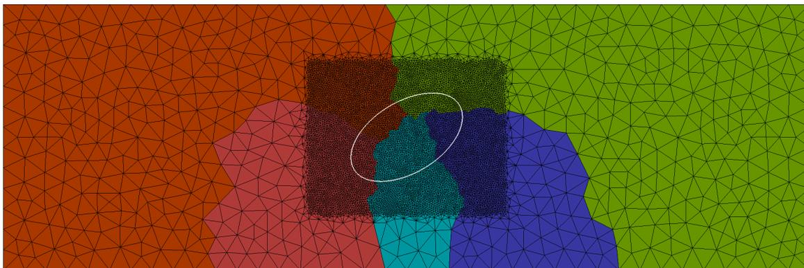
Figure 4.15: A vesicle in tank-treading simulation in the computational domain. The mesh has been added with its refinement around the vesicle. The sub domains associated to different processors are represented with different colors.
