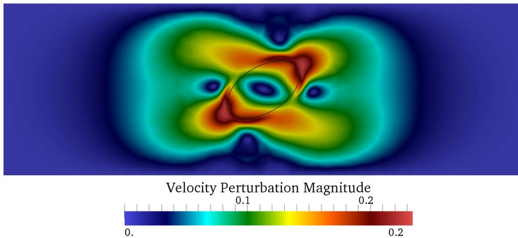
(b) Magnitude of the perturbation velocity  $|\mathbf{u} - \mathbf{u}_{\text{shear}}|$ . The perturbation field vanishes away from the vesicle. It is higher in the regions where the vesicle membrane forces the fluid to go in the opposite direction that the unperturbed one.
