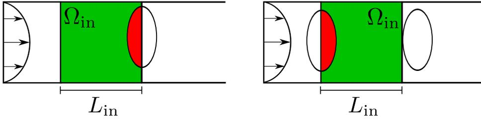
Figure 7.5: Scheme of the inlet of the bifurcation. The domain  $\Omega_{\text{in}}$  is represented in green. The area where  $(1 - H_\varepsilon(\phi)) \neq 0$  is represented in red. On the left hand side, the quantity  $A_{\text{in}}$  is too high for a new vesicle to be added. On the right hand side, the vesicle just exited the domain  $\Omega_{\text{in}}$ , this makes  $A_{\text{in}}$  vanishing, thus a new vesicle is added.
