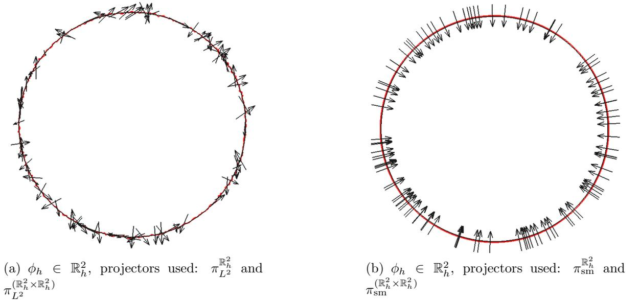
Figure 4.2: The iso 0 line of the level set field  $\phi_h$  is represented in black. The iso value 2 of the curvature  $\kappa_h$  is represented as the red line, and its gradient  $\mathbf{i}_h$  as black vectors randomly distributed on the curvature line.
