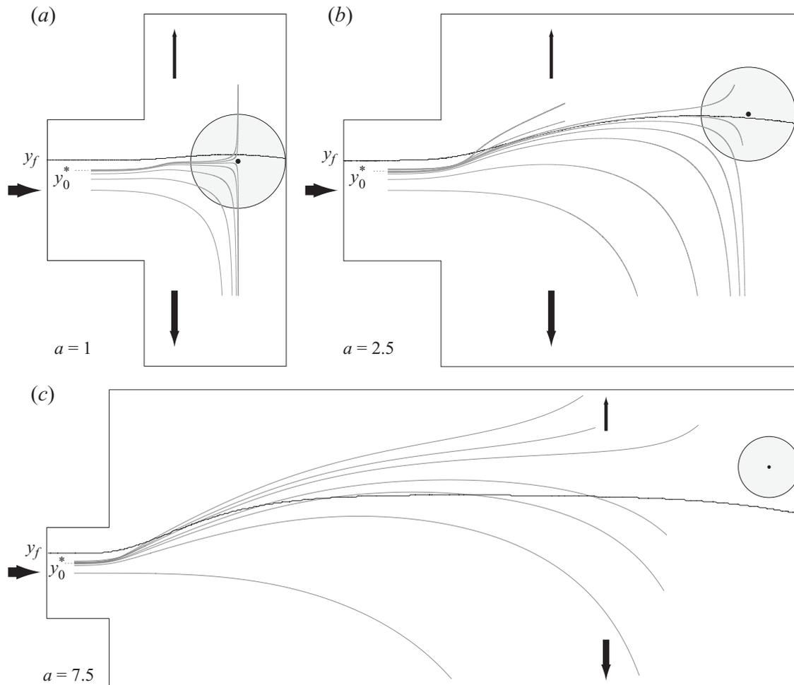
FIGURE 6. Comparison between fluid and particle trajectories in the vicinity of the bifurcation. Grey lines, some trajectories of an  $R=0.67$  particle when  $Q_1/Q_0=0.2$  for (a) branches of equal widths, (b) daughter branches 2.5 times wider than the inlet branch and (c) daughter branches 7.5 times wider than the inlet branch. The unperturbed fluid separating streamline starting at  $y = y_f$  is shown in black. The particle is shown approximately at its stagnation point.
