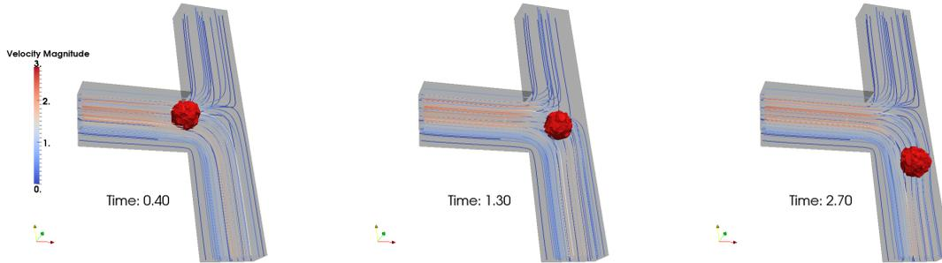
Figure 3.2: 3D simulation of the bifurcation problem. Some streamlines are represented on the figure and colored with the velocity magnitude  $|\mathbf{u}|$ . The area in which  $\mu = \mu_2$  is represented in red. This simulation has been run on a single processor which explains the rough grain of the particle.
