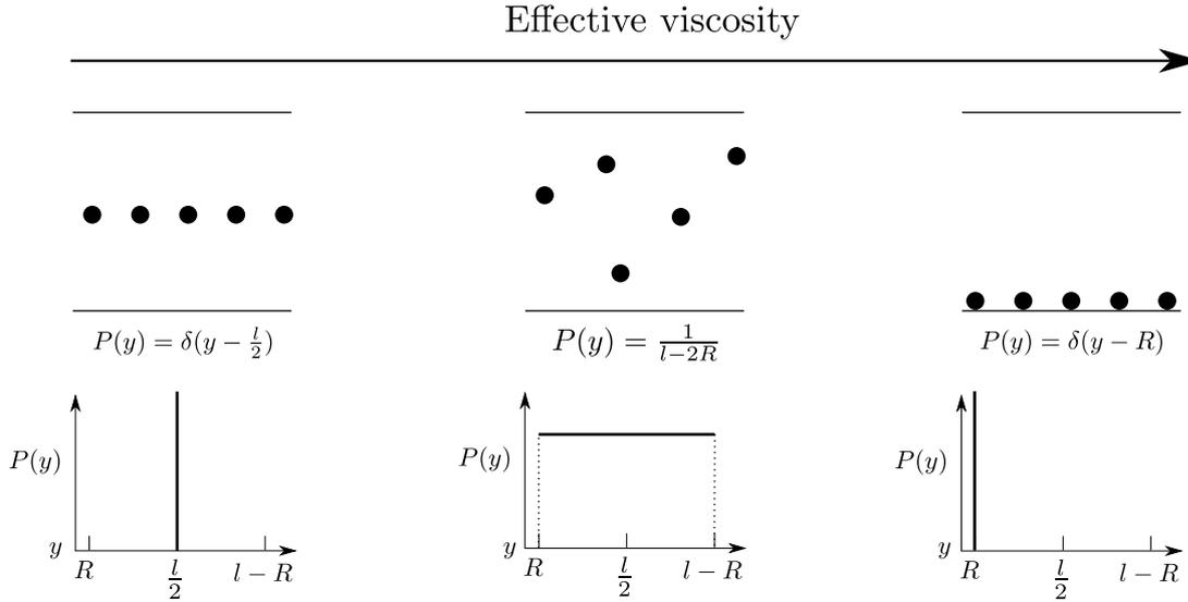
Figure 8.8: Three remarkable configurations at the points of view of the effective viscosity and their probability densities. The first and last one are respectively the configurations giving the lowest and highest effective viscosity. The middle one is the one often considered: a homogeneous suspension. In these schemes, the  $x$  direction has been shrunk for a better representation, but the particles should be separated of at least 5 radii to consider the suspension as dilute.
