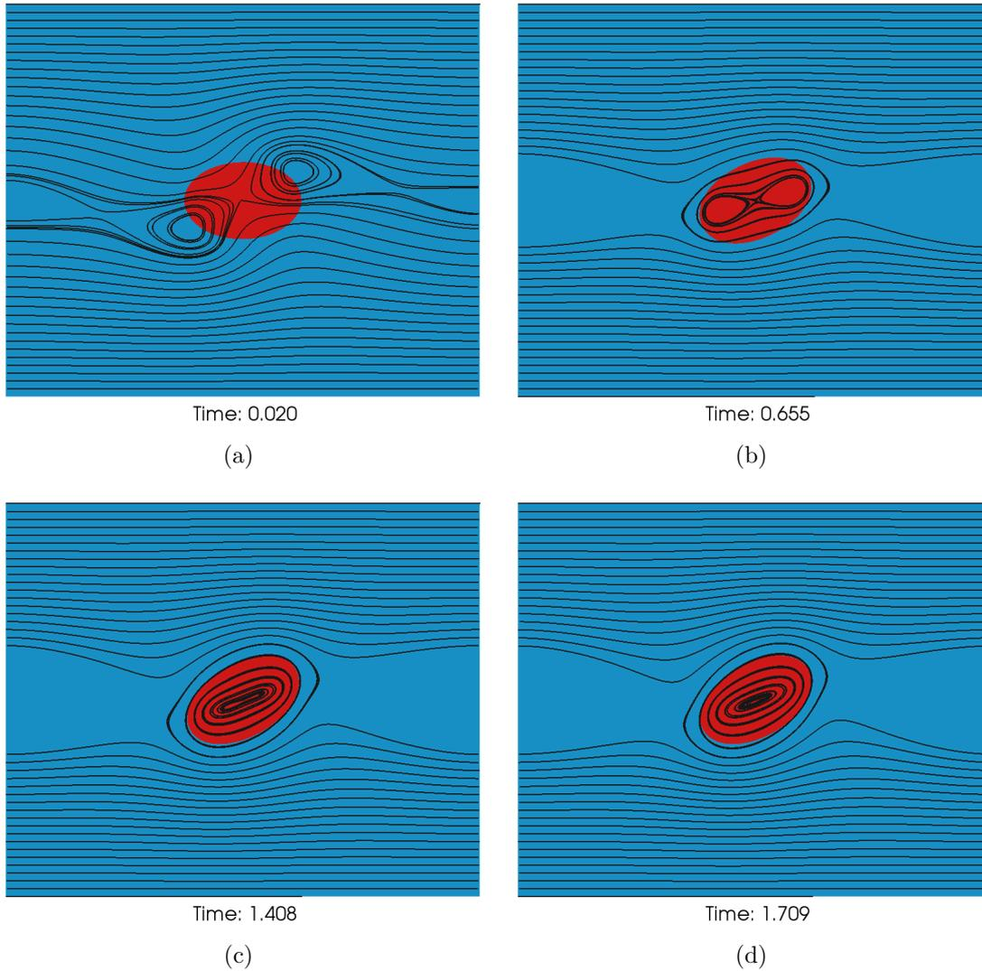
Figure 4.12: Vesicle in shear flow under tank-treading regime. The inside fluid of the vesicle (where  $\phi < 0$ ) is represented in red, whereas the outside fluid ( $\phi > 0$ ) is represented in blue. The streamlines are represented as black lines.
