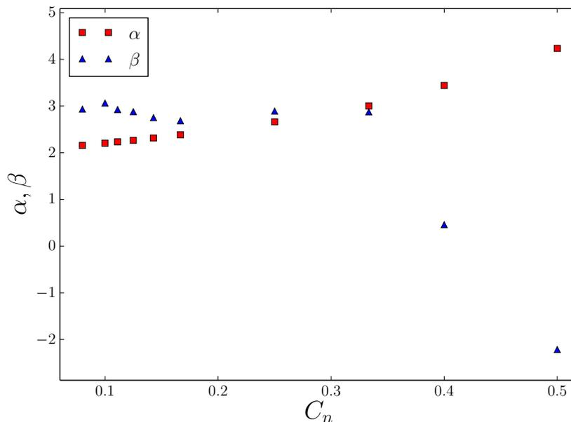
Figure 8.14: The coefficients of the fit of the viscosity curves as the one given in figure 8.13 for different confinement. The values of the  $\alpha$  coefficient are represented as red squares whereas the  $\beta$  values are blue triangles. One can see that the  $\alpha$  coefficient converges toward the Einstein's value for smaller confinement. The  $\beta$  factor decreases for stronger confinement and even becomes negative.
