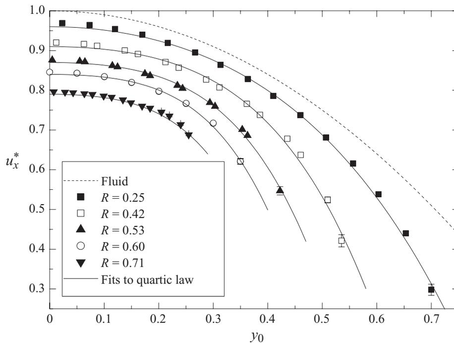
FIGURE 8. Some longitudinal velocity profiles  $u_x^*(y_0)$  for two-dimensional spheres of different radii  $R$  in the inlet channel, where a Poiseuille flow of velocity  $u_x(y) = 1 - y^2$  is imposed at infinity. The full lines show the fits by the quartic law  $u_x^*(y_0) = \alpha y_0^4 + \beta y_0^2 + \gamma$ .
