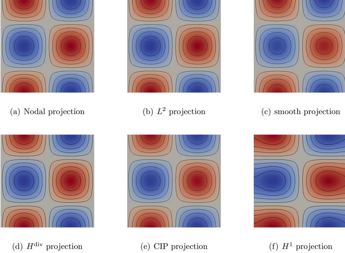
Figure 5.1: Results of the projection of  $f$  using different projectors. The color is the amplitude of the projected function  $f$ . The deepest red is 1, the deepest blue is -1. 10 iso values are reported in black.
