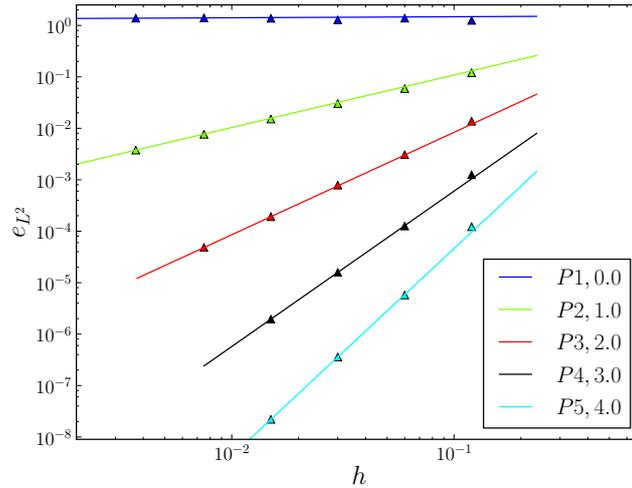
Figure 4.3:  $L^2$  error as a function of mesh size for different polynomial approximation order ( $\mathbb{P}^n$ ) using a  $L^2$  projection. The legend gives the polynomial approximation order of the initial level set field and the slope associated to the error.
