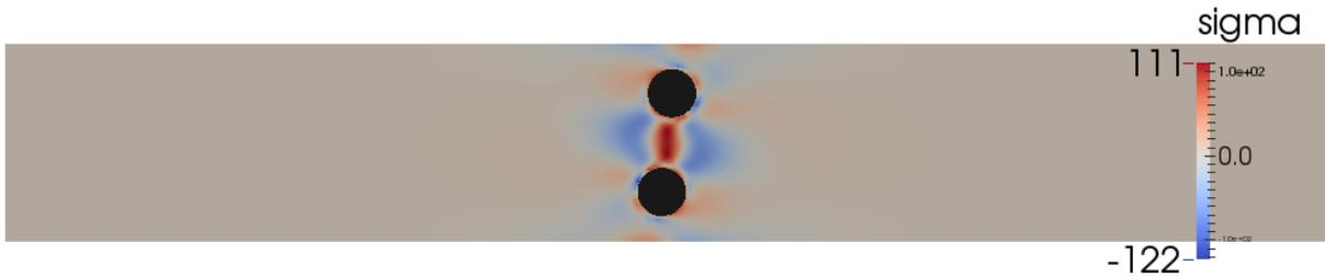
(c) The interaction is at its minimum when the particles are aligned along their  $y$  axis ( $\Delta x = 0$ ).Figure 8.10: The value of the field  $\sigma_{xy}^{2, \text{part}}$  for a confinement  $C_n = 0.1$  and a given  $\Delta y$  at three different  $\Delta x$ .
