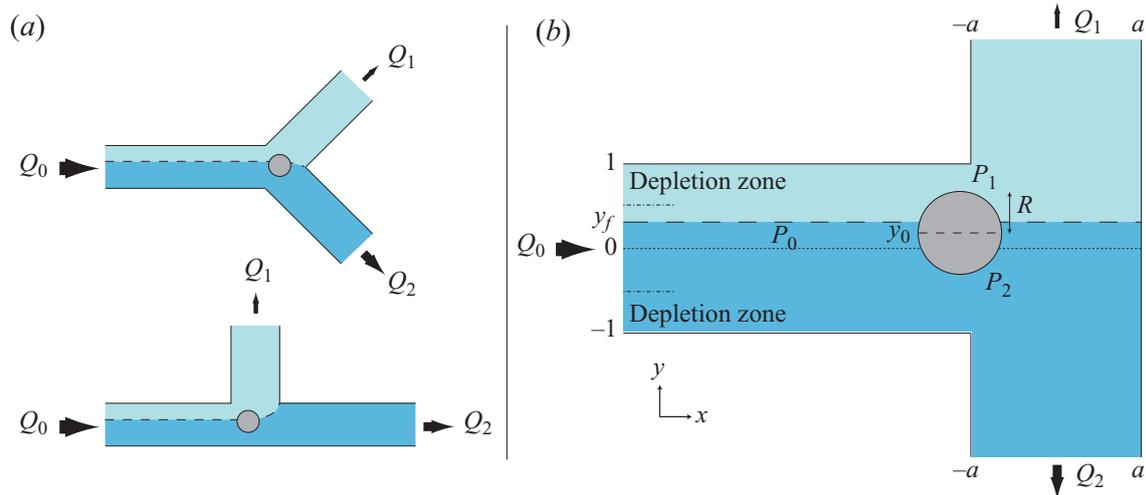
FIGURE 1. (Colour online) (a) The two Y-shaped geometries mainly studied in the literature. Here  $Q_1 < Q_2$  and the dashed line stands for the separating streamline between the flows that will eventually enter branches 1 and 2 in the absence of particles. (b) The T-bifurcation that is studied in this paper and also in Chien *et al.* (1985) in order to remove geometrical effects as much as possible.
