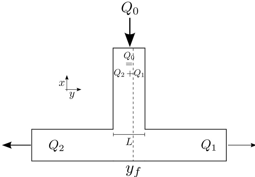
Figure 7.1: Bifurcation with a flow rate ratio  $\frac{Q_1}{Q_0} = 0.37$ . The separating line of fluid  $y_f$  is represented in dashed line. The fluid on the left of the separating line in the inlet channel goes in the left hand side branch and reciprocally for the right hand side.
