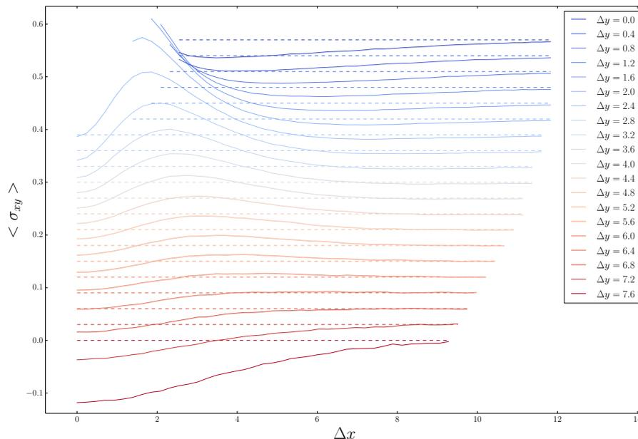
(a) 2D representation of the simulation of the contribution to the viscosity of a pair of particles. For each different  $\Delta y$ , the quantity  $\langle \sigma_{xy}^2 \rangle^{\text{part}}$  is measured for many  $\Delta x$ . The curves are represented with an offset to avoid their overlapping. A dashed line represents the value of the offset for each curve. The color represents the value of  $\Delta y$  for each curve which are reported in the legend.
