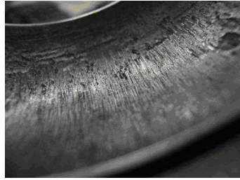
Figure 1.4: Outer ring ball damaged by fretting in temperature
