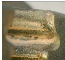
Figure 1.3: Contact zone of the disk in the TuHP subjected to fretting in temperature
