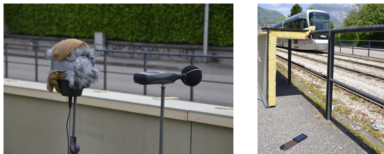
Figure 8.6: Devices used in the measurements. Left: B&K type 2250 sound level meter and binaural head. Right - cellphone LG P970 used as an auxiliary microphone for speed measurement.
