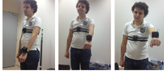
Figure 6.6: Experimental Scenarios 2 (left), 3 (middle) and 4 (right): On-body ranging over the chest-wrist link in direct LOS visibility, for different body attitudes.
