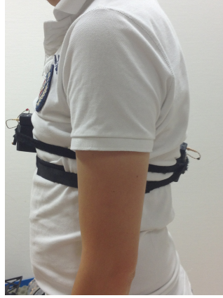
Figure 6.10: Experimental Scenario 5: On-body ranging over a static chest-back link, under systematic NLOS conditions.
