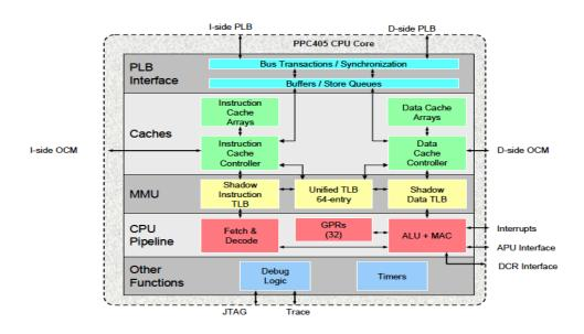
Figure 3.3: Block diagram of PowerPC processor: source [55]
