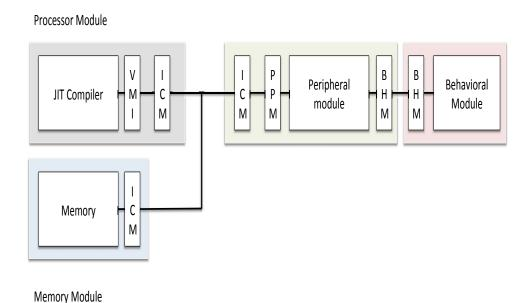
Figure 4.2: Communication of OVP interfaces
