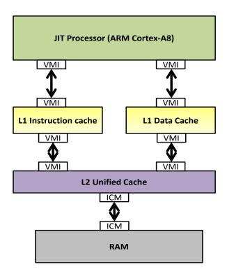
Figure 4.3: Cortex-A8 interface implementation
