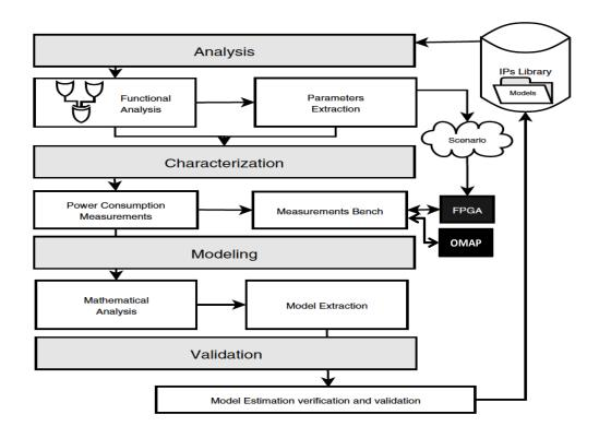
Figure 3.5: Power characterization and modeling methodology framework: source [41]
