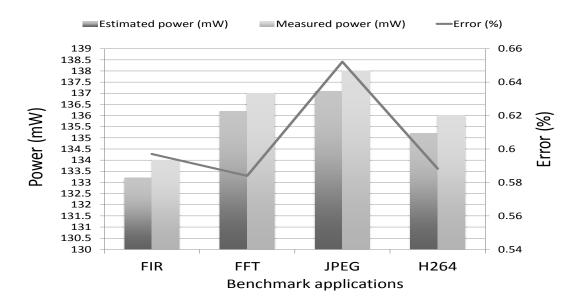
Figure 3.23: Validation of the power model for ARM9
