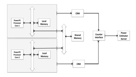
Figure 5.12: Dual core PowerPC platform
