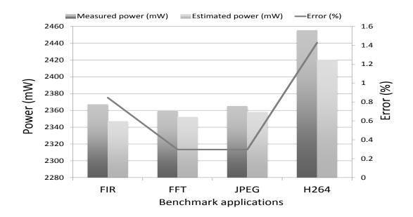
Figure 3.24: Validation of the power model for PowerPC
