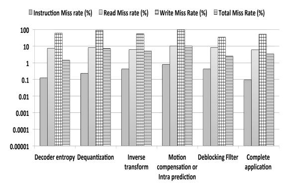
Figure 5.6: Cache miss rate for the H.264 application (ARM9 at 120 MHz)
