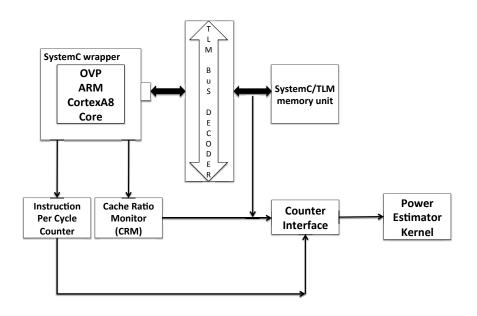
Figure 5.3: Mono-processor platform of ARM Cortex-A8
