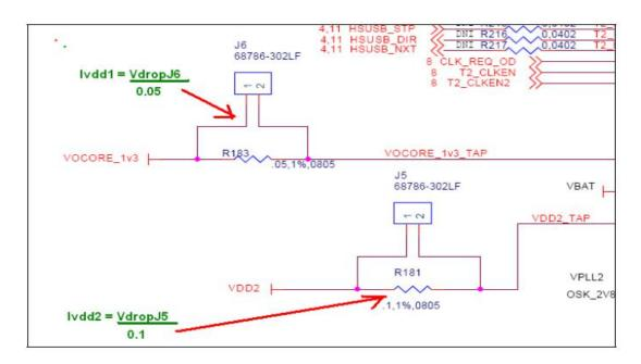
Figure 3.10: Power measurement jumpers for the OMAP3530 platform
