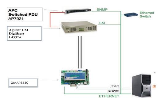
Figure 3.7: Measurement environment for OMAP3530 and OMAP5912
