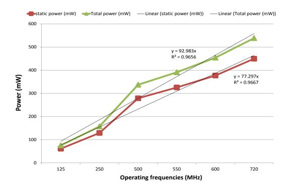
Figure 3.14: Power consumption cost according to the change in frequency cation.
