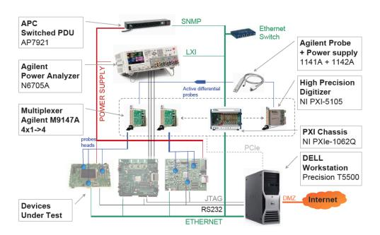
Figure 3.6: Fully automated test bench for current/voltage measurement
