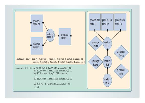
Figure 2.11: Mapping network: source [22]
