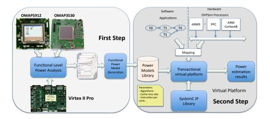
Figure 5.1: Power estimation flow
