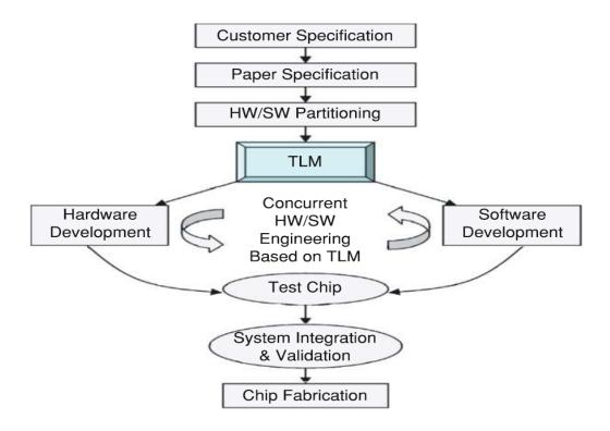
Figure 2.4: TLM design flow: source [46]
