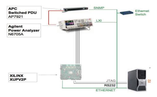
Figure 3.11: Measurement environment for Virtex-II Pro FPGA
