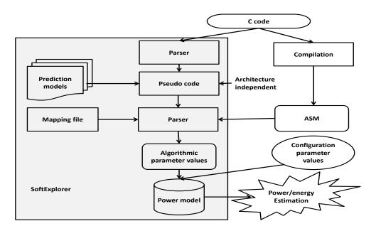
Figure 2.9: SoftExplorer power estimation flow: source [59]
