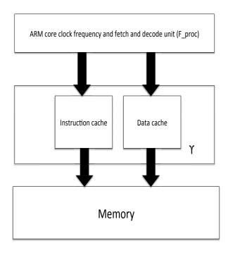
Figure 3.15: Main functional blocks of ARM9 processor
