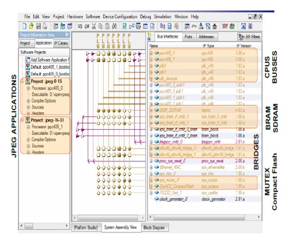
Figure 3.16: Xilinx EDK 10.1 design for two PowerPC processors with shared memory
