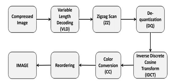
Figure 4.14: JPEG decoder flow
