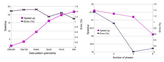
Figure 4.17: Power estimation error and speedup according to the data pattern Figure 4.18: Power estimation error and granularity speedup according to the number of phases
