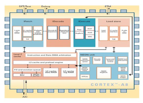
Figure 3.1: Block diagram of ARM Cortex-A8 processor : source [16]
