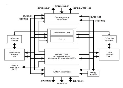
Figure 3.2: Block diagram of ARM9TDMI processor : source [17]
