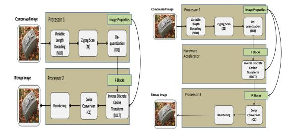
Figure 4.15: JPEG decoding process Figure 4.16: JPEG decoding process with 2 processors and hardware accelerator
