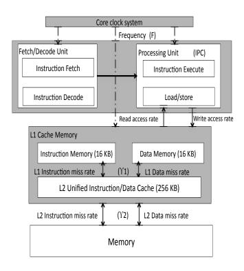
Figure 3.12: Main functional blocks of ARM Cortex-A8 processor
