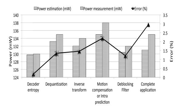
Figure 5.7: Power estimation accuracy for the H.264 application using ARM9 at  $120~\mathrm{MHz}$
