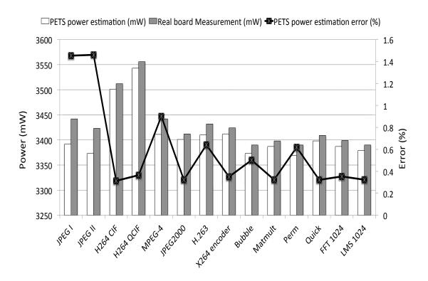
Figure 5.14: Power estimation of homogeneous two PowerPC multiprocessor architecture  $\,$
