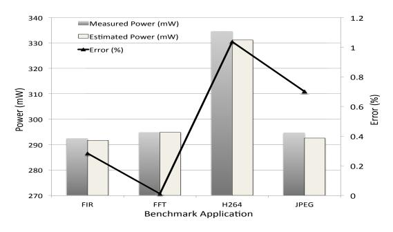
Figure 3.22: Validation of the power model for ARM Cortex-A8
