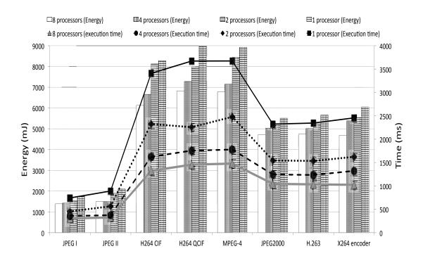
Figure 5.15: Energy estimation according to the number of processors using PowerPC
