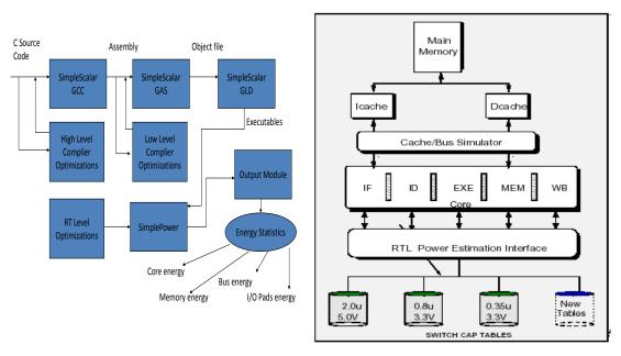
Figure 2.6: Complier of SimplePower tool
