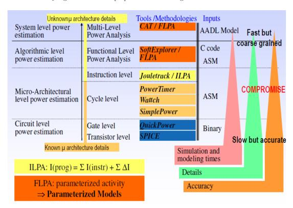
Figure 2.5: Power modeling methodologies and tools according the abstraction levels  $\frac{1}{2}$
