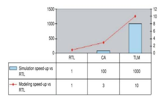
Figure 2.3: TLM speed-up in terms of modeling efforts and simulation speed : source [46]
