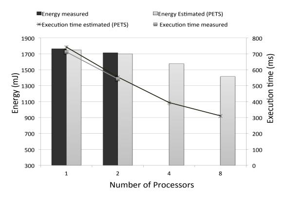
Figure 5.13: Execution time and energy variation according to the number of processors
