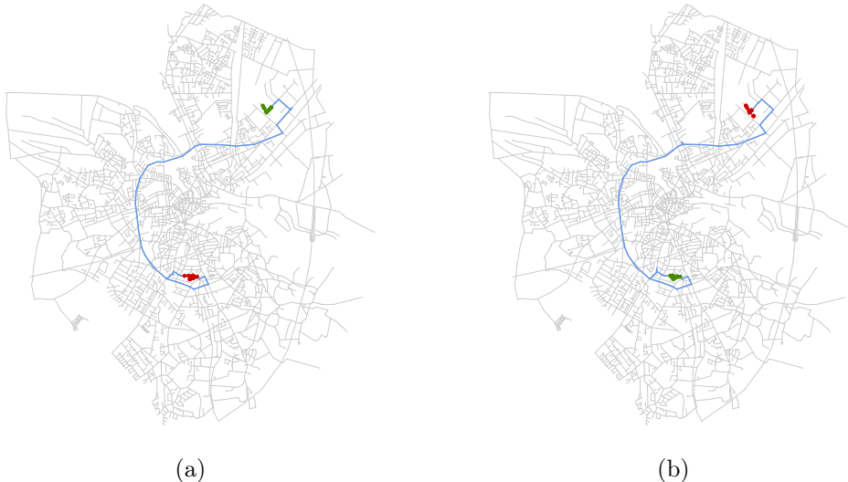
Figure 1.4 – Example of two inverted clusters of trajectories. The departure area of one cluster (depicted in green) is the destination area of the other cluster (in red) and vice versa.
