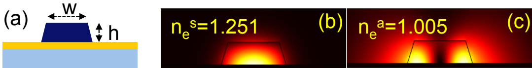
Figure 4.3: (a) Opto-geometrical parameters for the finite-element analysis of an un-doped DMI waveguides, W = 900\text{nm} , h = 400\text{nm} (see Fig. 4.3(a)), n_{\text{PMMA}} = 1.489 , n_{\text{Au}} = 0.57 + i11.7 for a wavelength of \lambda_o = 1580\text{nm} . The trapezoidal shaped cross-cut of the DLSPPW accounts for the undercut of the vertical side-walls produced by PMMA processing. (b) (resp. (c)) Spatial distribution of the guided power for the fundamental symmetric (resp. higher-order anti-symmetric) DLSPPW mode.
